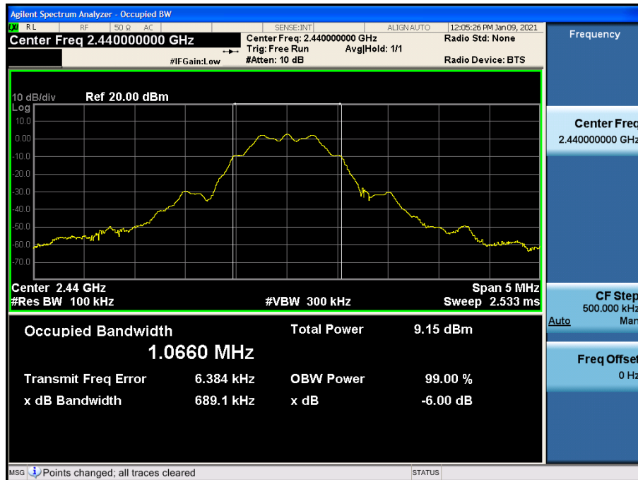
6 dB Bandwidth plot (Mid-CH 19)
