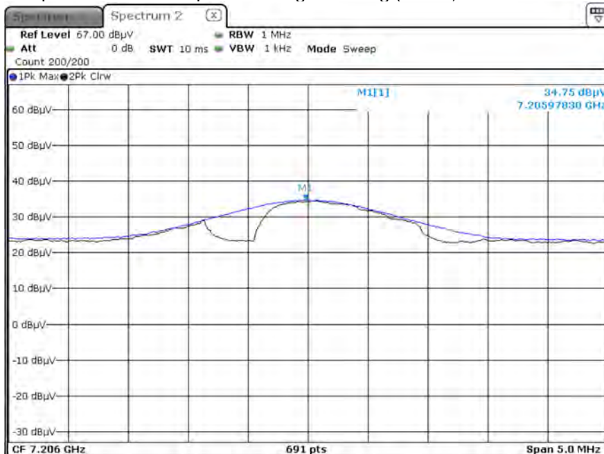
Radiated Spurious Emissions plot – Average Reading (GFSK, Ch.0 3rd Harmonic, Y-H)
