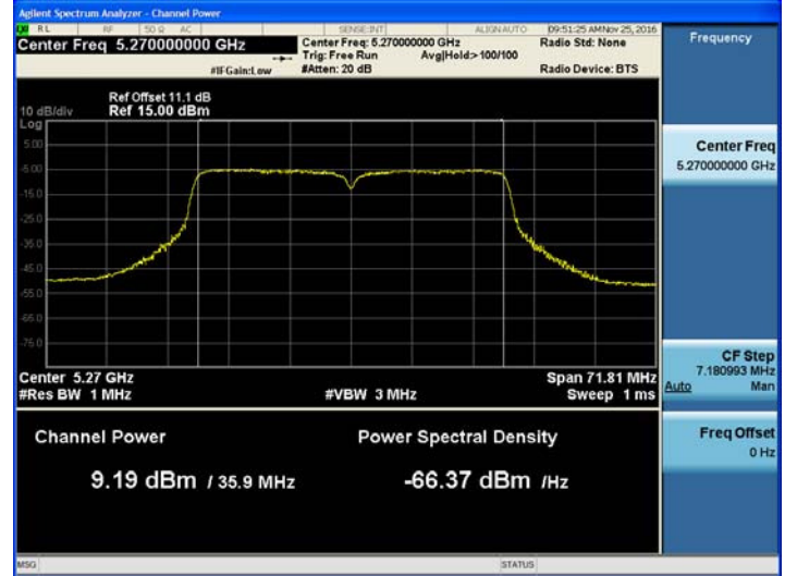
802.11ac_VHT40 UNII 3 BAND Average Power (5755 MHz ~5795 MHz) CH 159 MCS3
