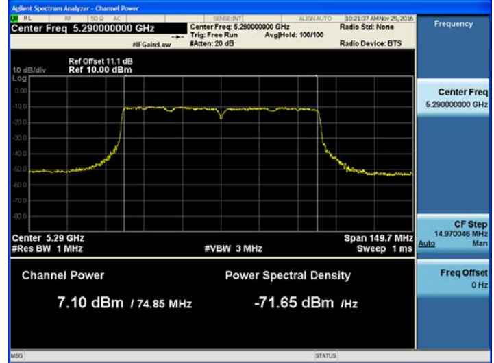
802.11ac_VHT80 UNII 3 BAND Average Power (5775 MHz) CH 155 MCS3
