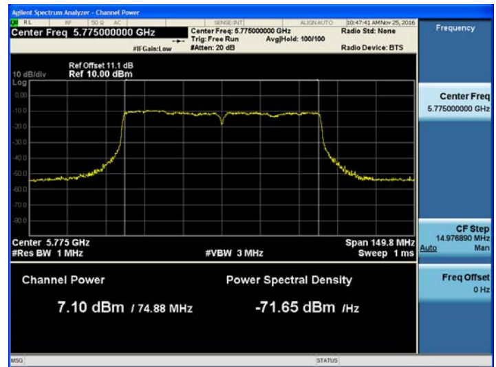
802.11ac_VHT80 UNII 3 BAND Average Power (5775 MHz) CH 155 MCS3
