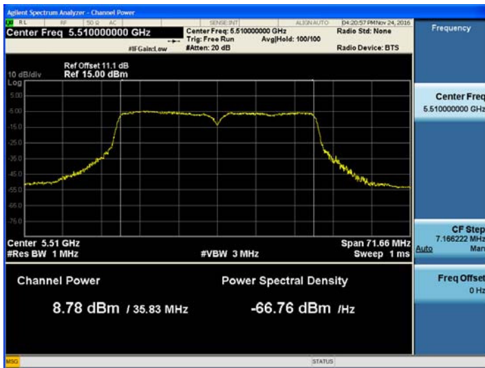
802.11n_HT40 UNII 2C BAND Average Power (5510 MHz ~5670 MHz) CH 102 MCS5
