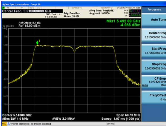
802.11n_HT40 UNII 2C BAND PSD CH 102
