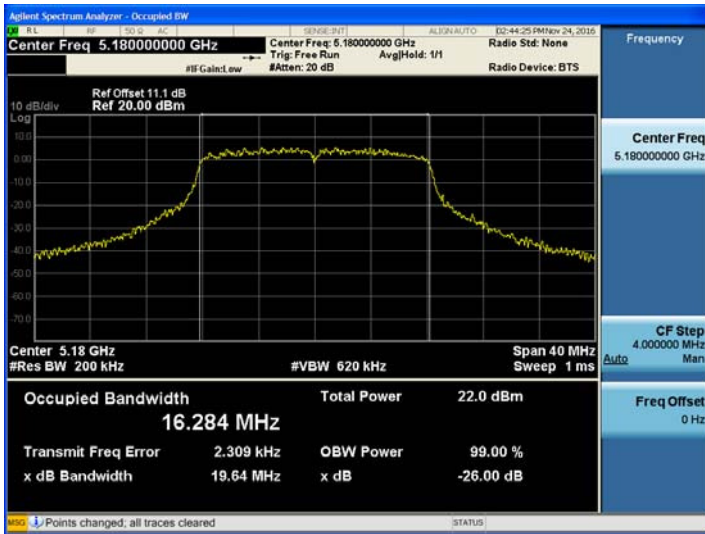
802.11a UNII 2C BAND 26dB Bandwidth (CH140)
