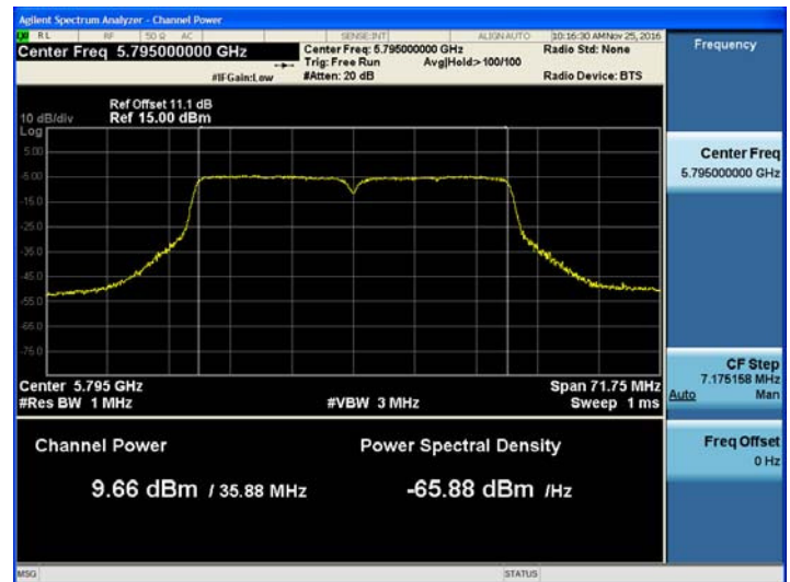
802.11ac_VHT40 UNII 3 BAND Average Power (5755 MHz ~5795 MHz) CH 159 MCS3
