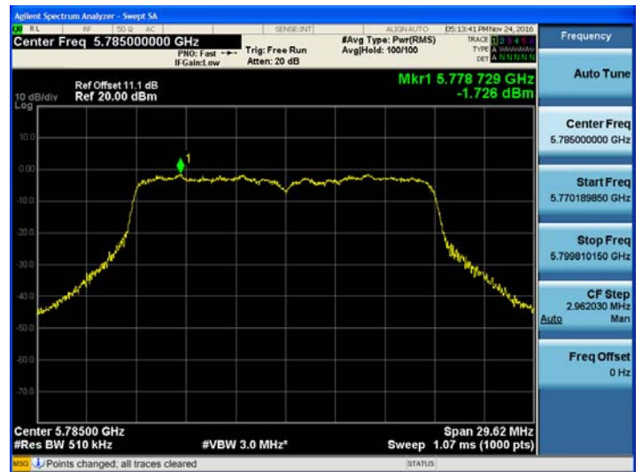
802.11ac_VHT20 UNII 3 BAND PSD CH 157
