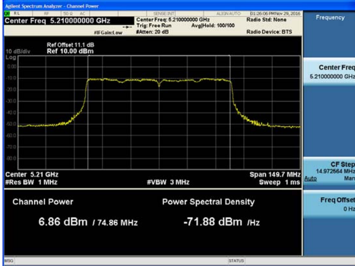
802.11ac_VHT80 UNII 2C BAND Average Power (5530 ~ 5610 MHz) CH 106 MCS3
