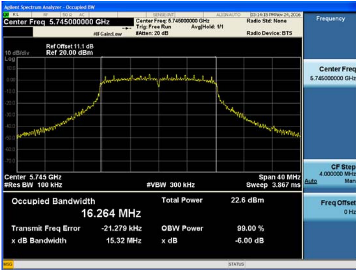
802.11ac_VHT20 UNII 3 BAND 6dB Bandwidth(CH.165)
