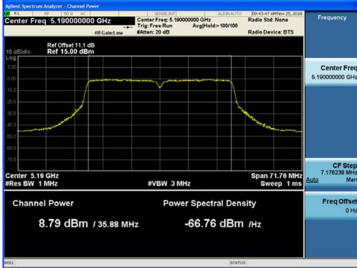
802.11ac_VHT40 UNII 2C BAND Average Power (5510 MHz ~5670 MHz) CH 102 MCS3
