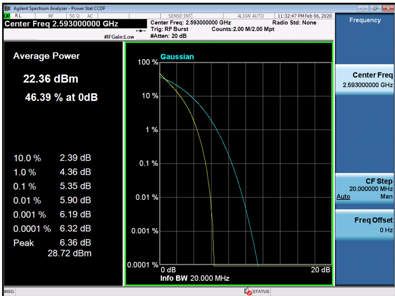
BAND 41. PAR Plot (20M BW\_Ch.40620\_16QAM\_RB100\_0)
