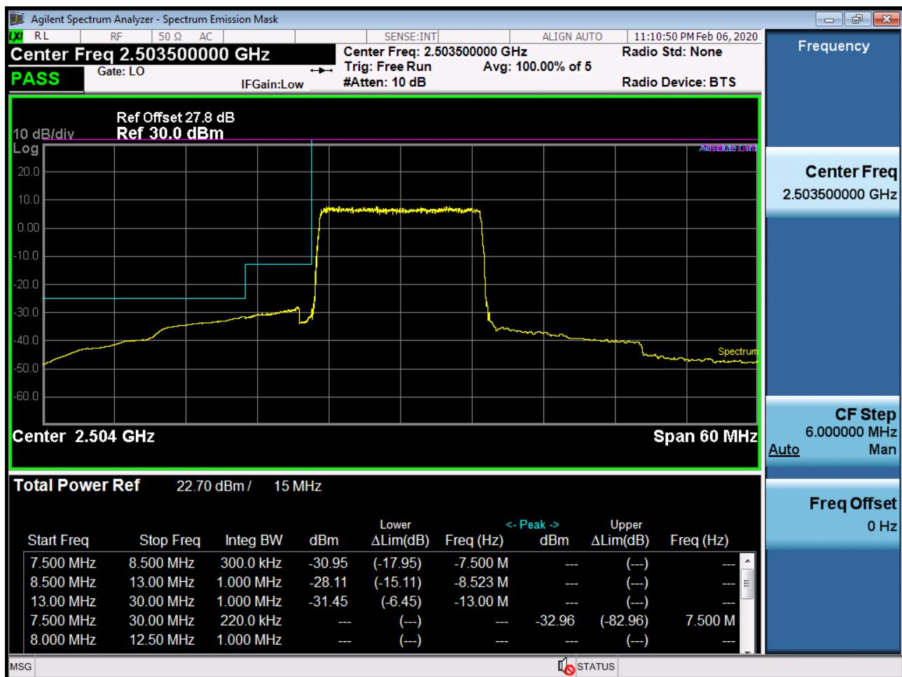
BAND 41. Low Channel Edge Plot (15 MHz Ch.39725 QPSK\_RB1\_Offset 0)-2
