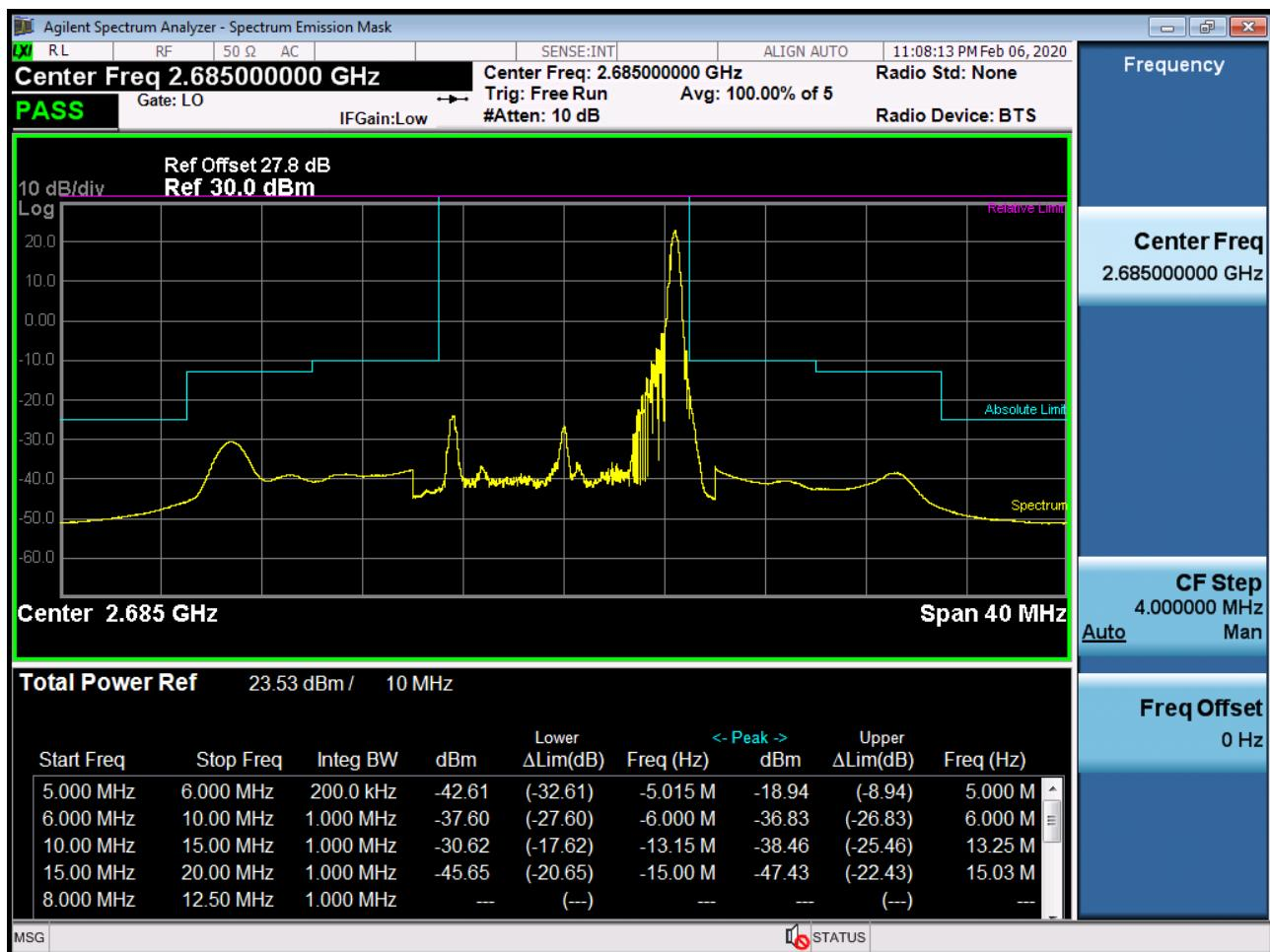
BAND 41. High Channel Edge Plot (10 MHz Ch.41540 QPSK\_RB50\_Offset 0)
