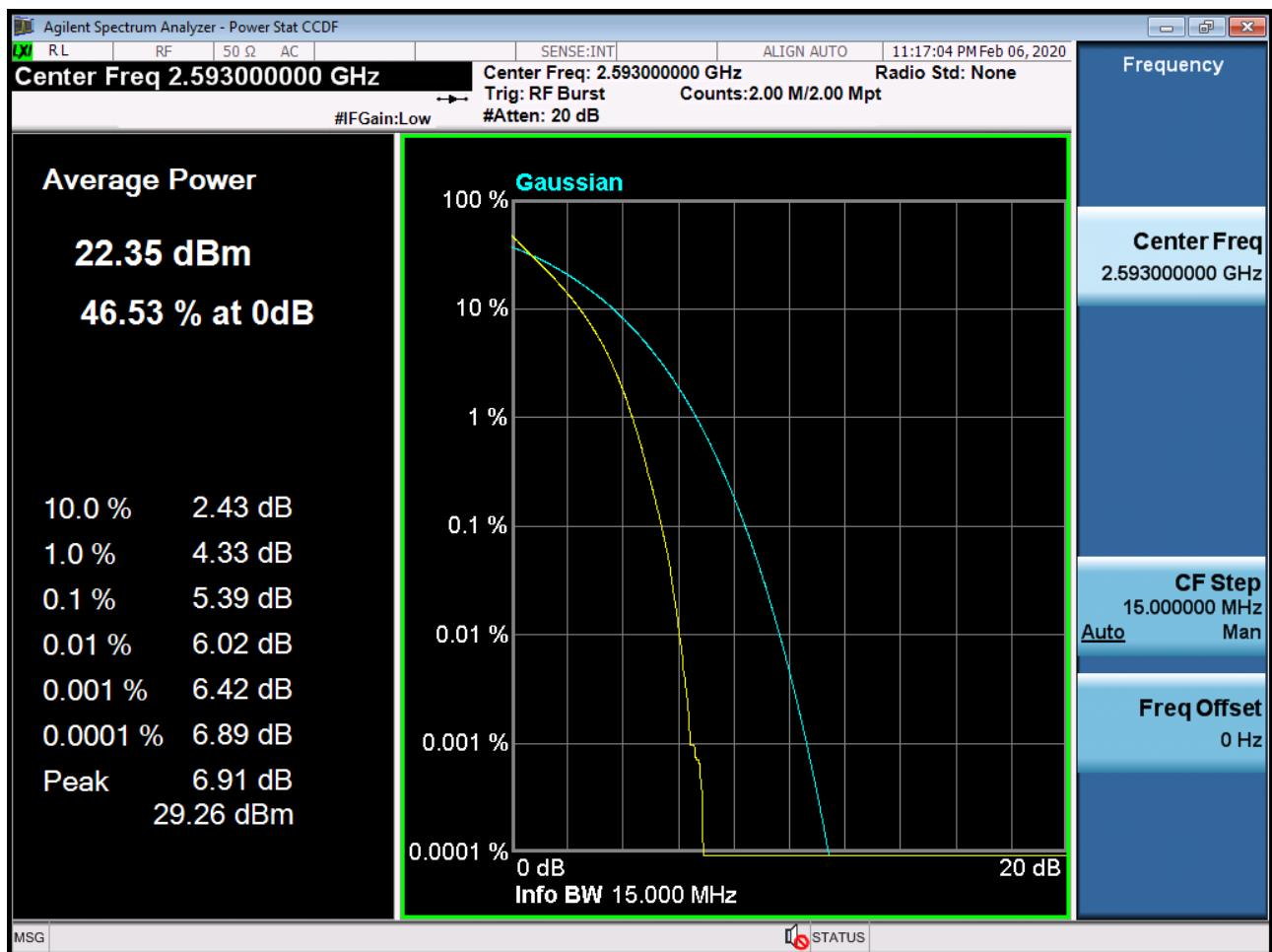
BAND 41. PAR Plot (15M BW\_Ch.40620\_16QAM\_RB75\_0)
