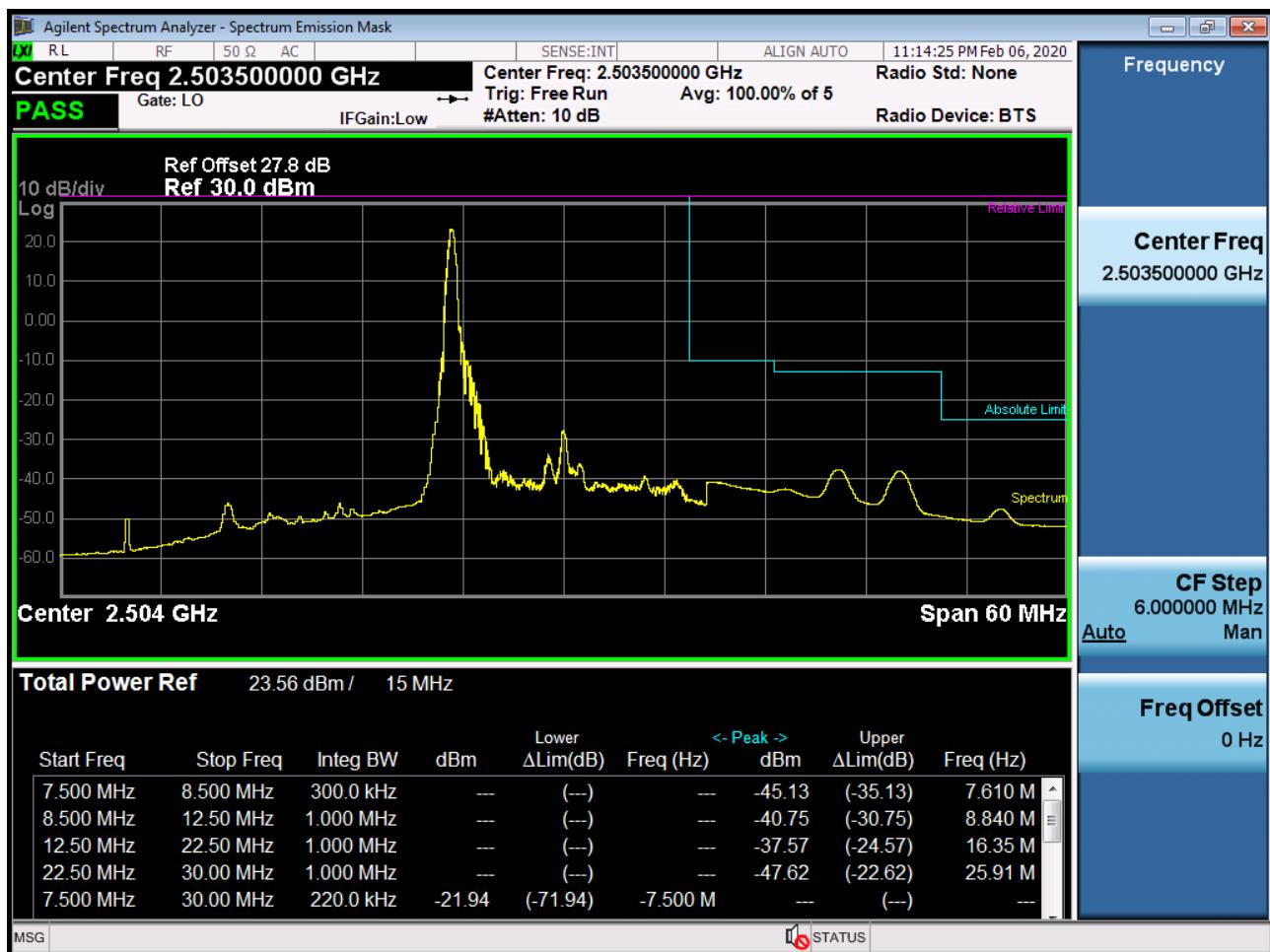
BAND 41. Low Channel Edge Plot (15 MHz Ch.39725 QPSK\_RB75\_Offset 0)-2
