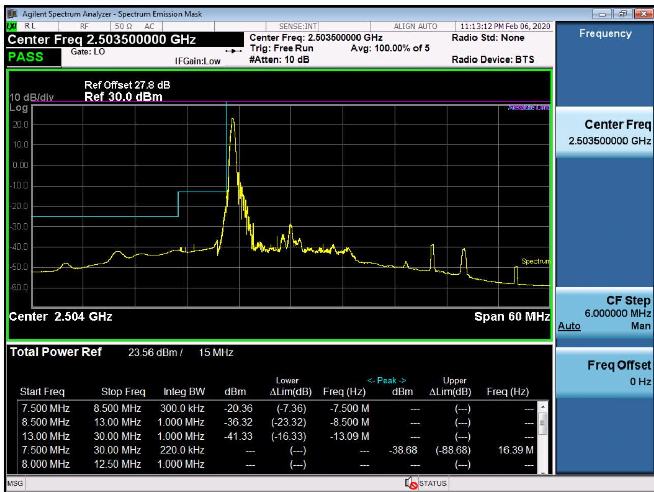
BAND 41. Low Channel Edge Plot (15 MHz Ch.39725 QPSK RB 75, Offset 0)-1
