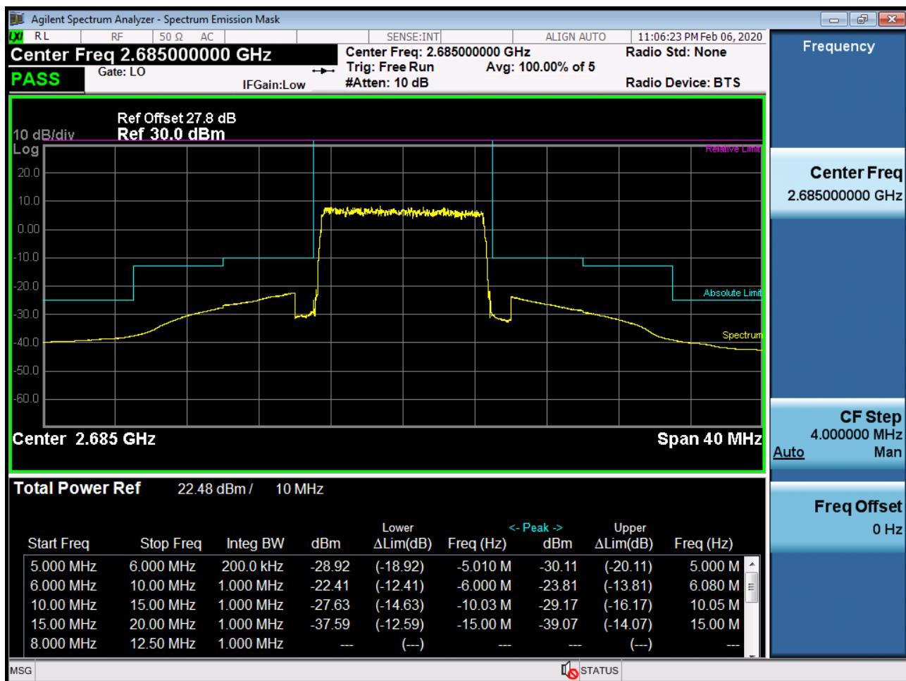
BAND 41. Low Channel Edge Plot (15 MHz Ch.39725 QPSK RB 1, Offset 0)-1
