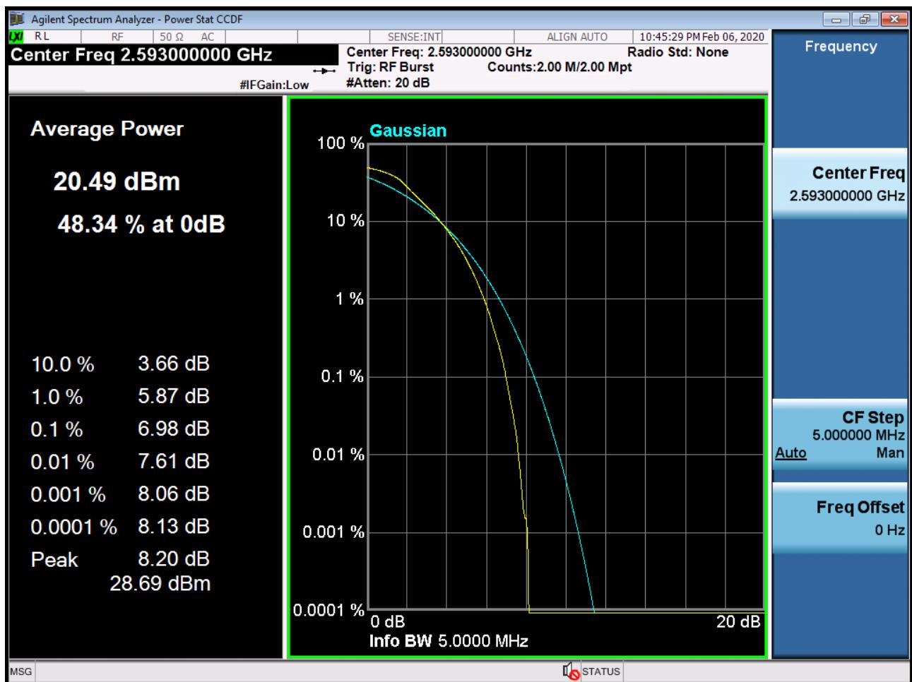
BAND 41. PAR Plot (5M BW\_Ch.40620\_16QAM\_RB25\_0)
