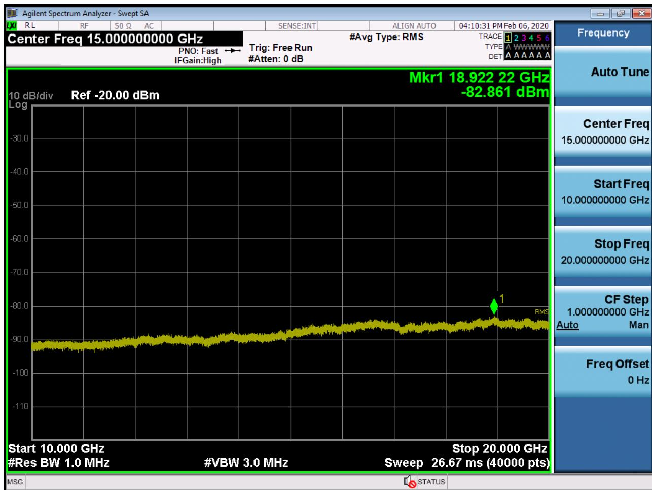
BAND 2. Conducted Spurious\_1 (19193ch\_1.4MHz\_QPSK\_RB 1\_0)
