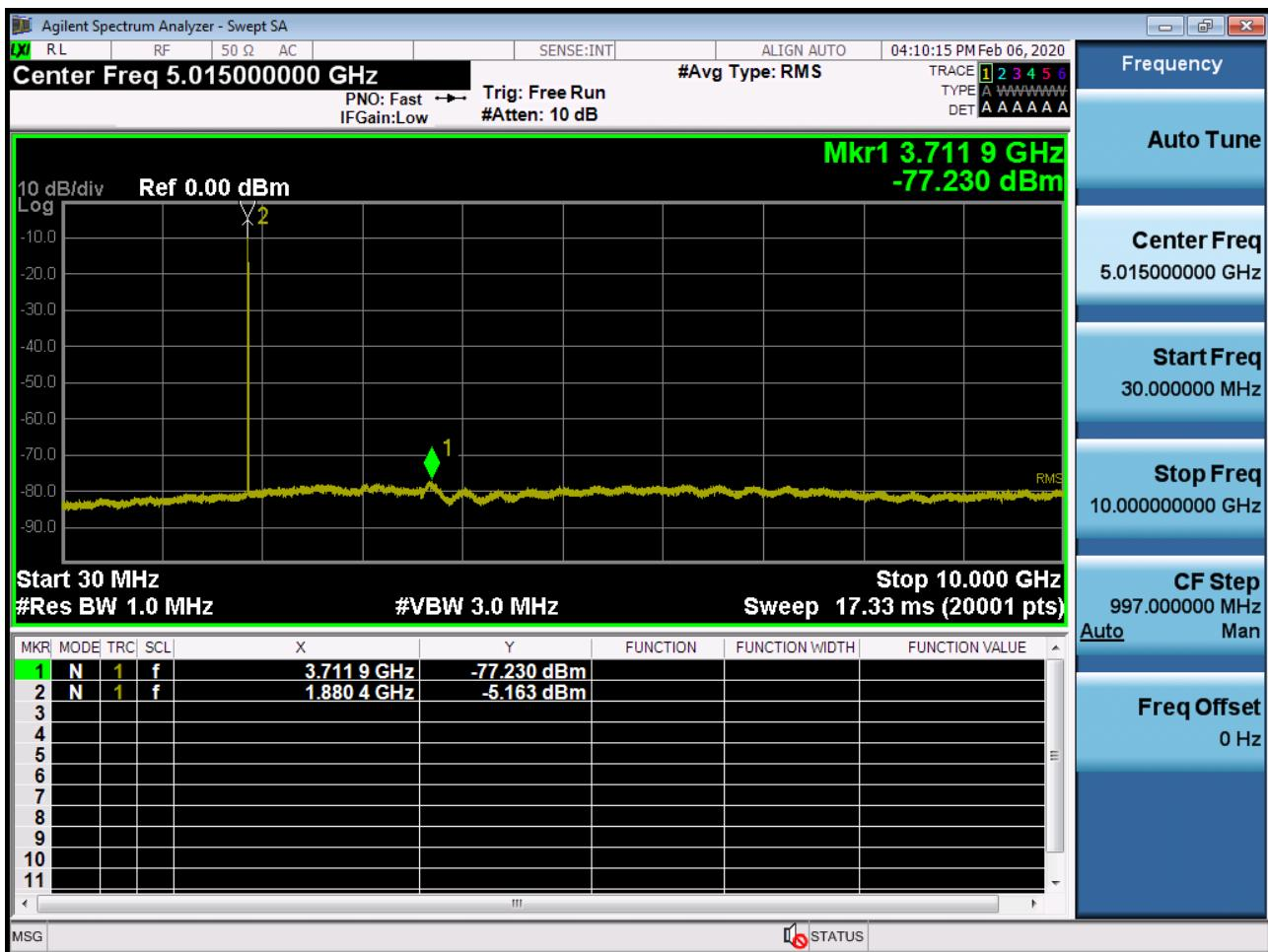
BAND 2. Conducted Spurious\_2 (18900ch\_1.4MHz\_QPSK\_RB 1\_0)
