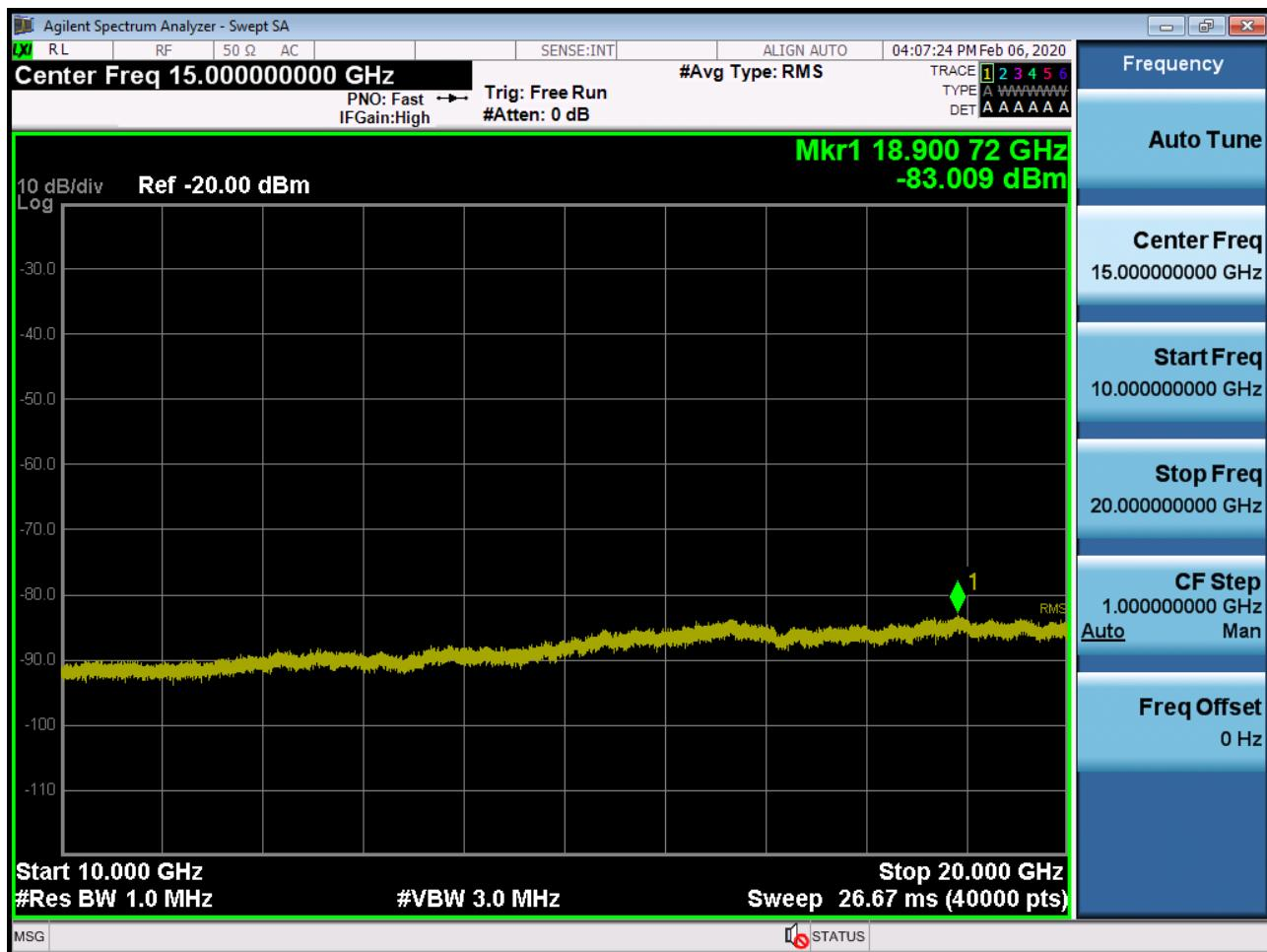
BAND 2. Conducted Spurious\_1 (18900ch\_1.4MHz\_QPSK\_RB 1\_0)
