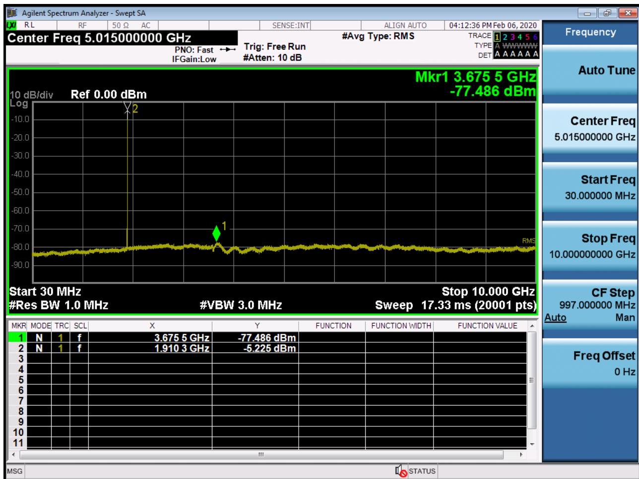
BAND 2. Conducted Spurious\_2 (19193ch\_1.4MHz\_QPSK\_RB 1\_0)
