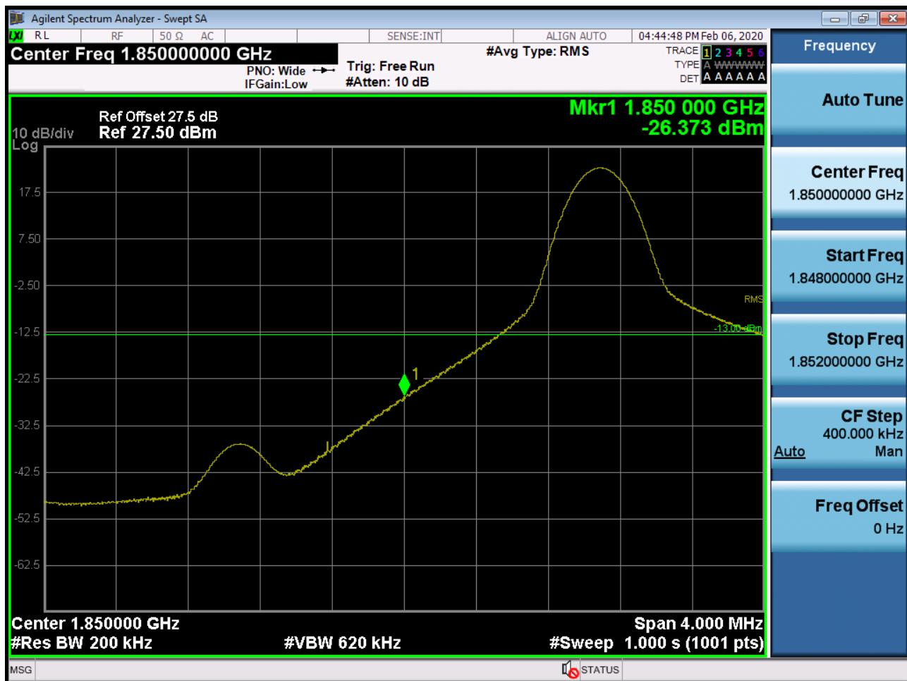
BAND 2. Lower Band Edge Plot (20M BW Ch.18700 QPSK\_RB100\_Offset 0) -2
