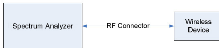
Figure 7-1. Test Instrument & Measurement Setup
