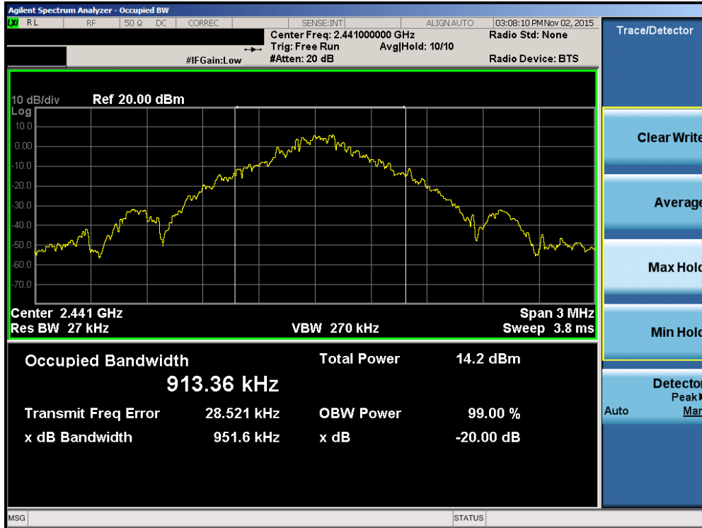
Plot 7-2. 20dB Bandwidth Plot (Bluetooth, 1Mbps – Ch. 39)
