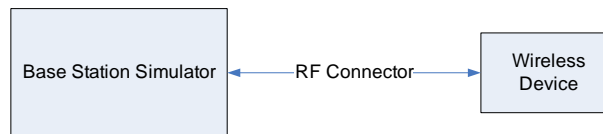
Figure 9-1 Power Measurement Setup
