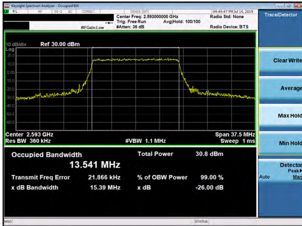
Plot 7-13. Occupied Bandwidth Plot (Band 41 - 15.0MHz QPSK - Full RB Configuration)
