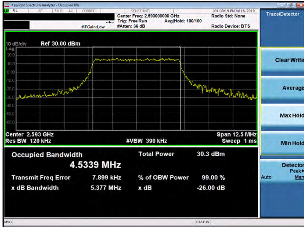
Plot 7-9. Occupied Bandwidth Plot (Band 41 - 5.0MHz QPSK - Full RB Configuration)
