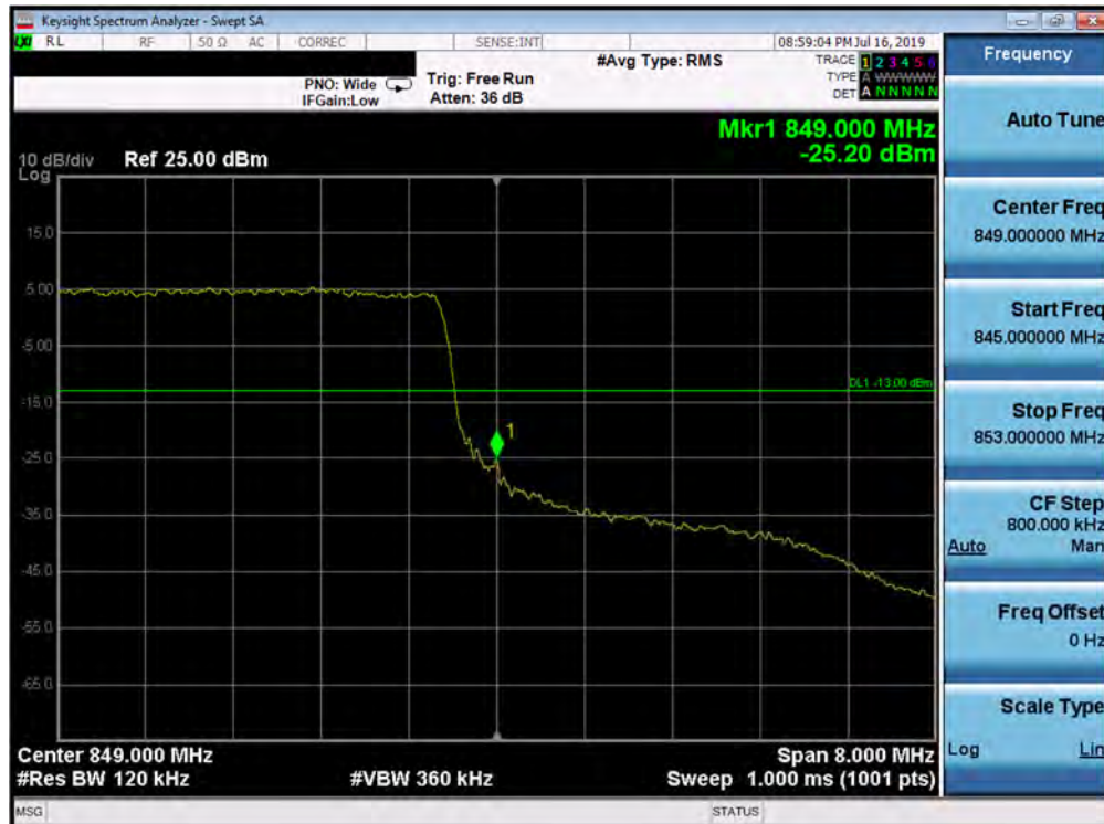
Plot 7-42. Upper Band Edge Plot (Band 5 - 10.0MHz QPSK - Full RB Configuration)
