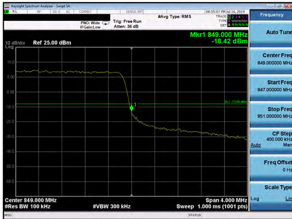
Plot 7-38. Upper Band Edge Plot (Band 5 - 3.0MHz QPSK - Full RB Configuration)
