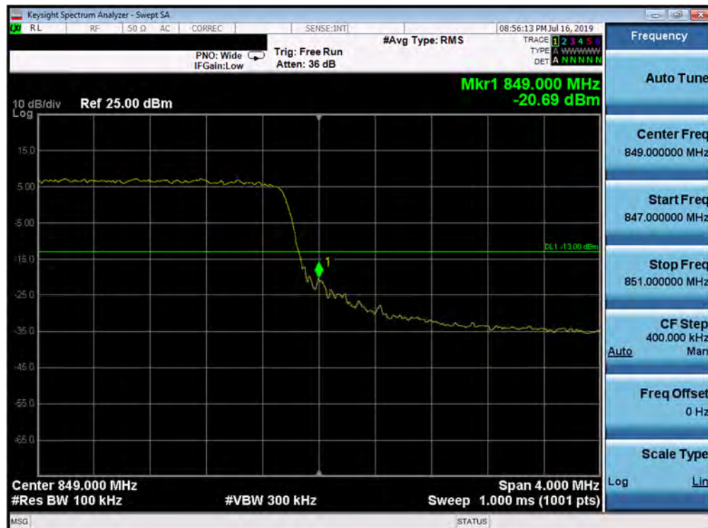
Plot 7-40. Upper Band Edge Plot (Band 5 - 5.0MHz QPSK - Full RB Configuration)
