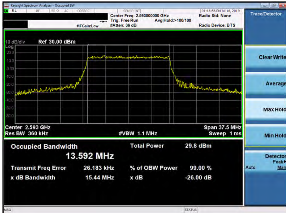
Plot 7-14. Occupied Bandwidth Plot (Band 41 - 15.0MHz 16-QAM - Full RB Configuration)
