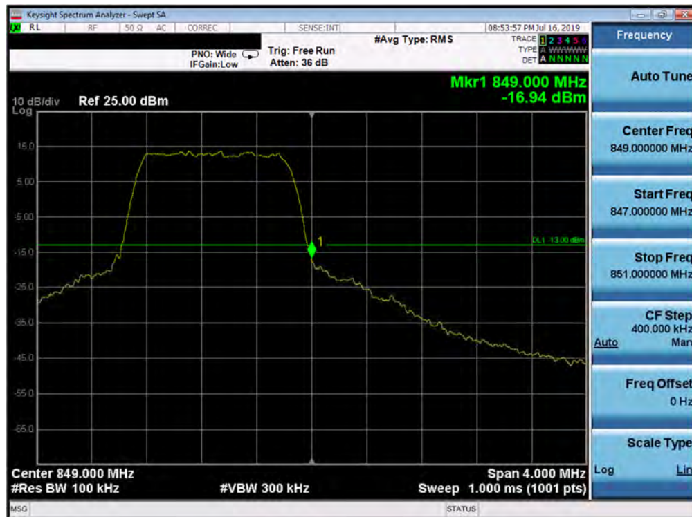
Plot 7-36. Upper Band Edge Plot (Band 5 - 1.4MHz QPSK - Full RB Configuration)
