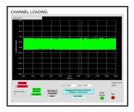
The level of traffic loading on the channel by the EUT is 36.036%.
