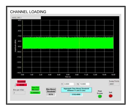
The level of traffic loading on the channel by the EUT is 33.504%.
