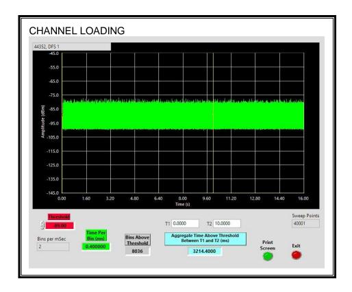
The level of traffic loading on the channel by the EUT is 32.144%.
