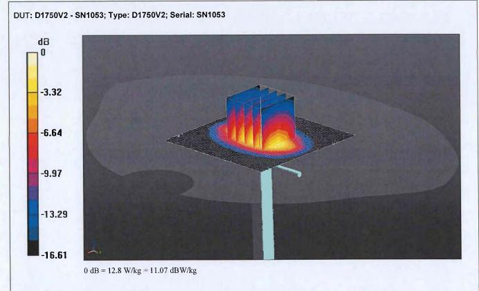
Communication System: UID 0, CW (0); Frequency: 1750 MHz; Duty Cycle: 1:1
