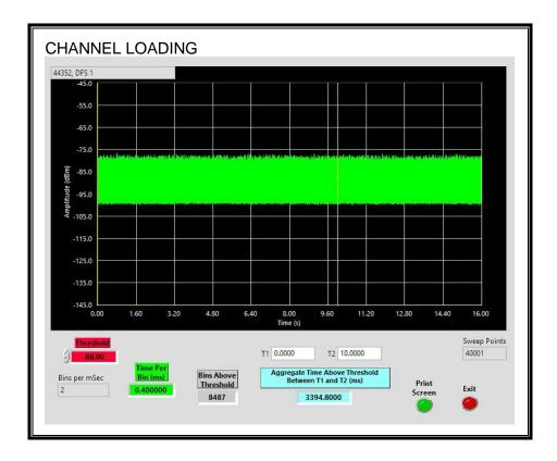
The level of traffic loading on the channel by the EUT is 33.948%.
