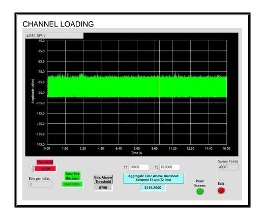
The level of traffic loading on the channel by the EUT is 35.192%.
