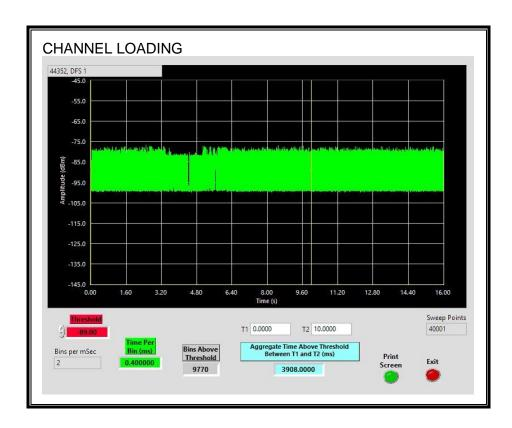
The level of traffic loading on the channel by the EUT is 39.08%.
