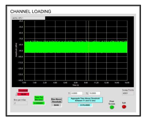
The level of traffic loading on the channel by the EUT is 33.784%.
