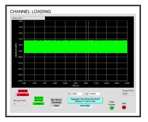
The level of traffic loading on the channel by the EUT is 31.872%.
