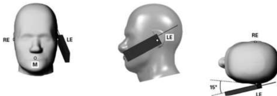
Figure 6.5. Tilt 15^\circ position of the wireless device
