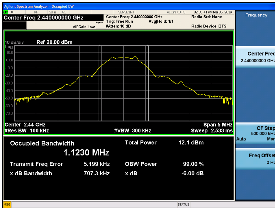
6 dB Bandwidth plot (Mid-CH 19)
