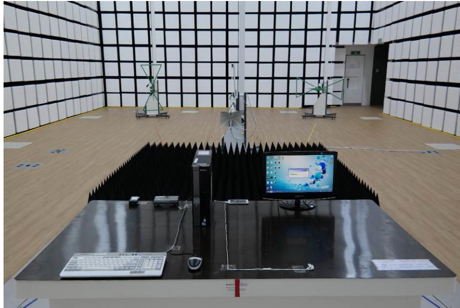
[ Radiated Disturbance for Above 1 GHz – Front ]
