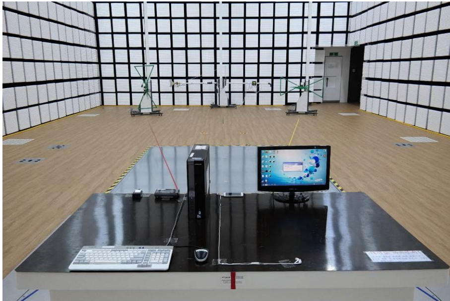
[ Radiated Disturbance for Below 1 GHz – Front ]
