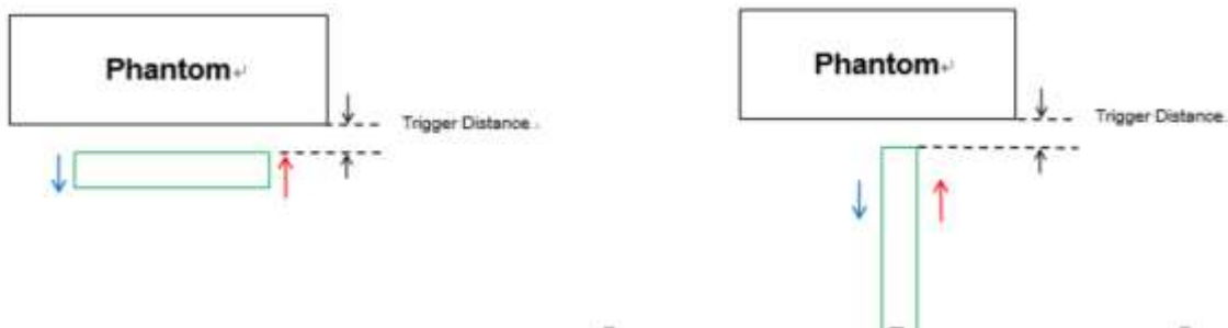
Proximity Sensor Trigger Distance Assessment KDB 616217 D04§6.2
