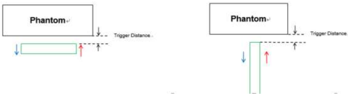
Proximity Sensor Trigger Distance Assessment KDB 616217 D04§6.2
