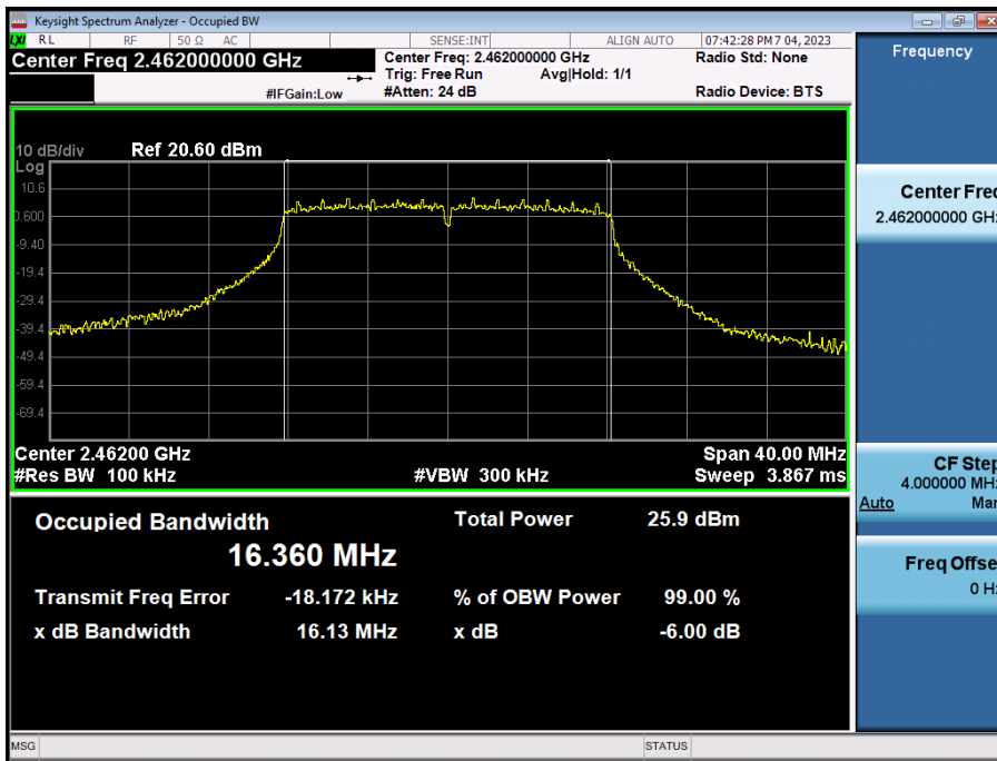
6 dB Bandwidth plot (802.11g-CH 11)
