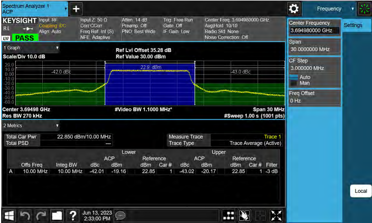
Sub6 n48. Adjacent Channel Leakage Ratio(ACLR) Plot (10 MHz Ch.646332 BPSK RB 24, Offset 0)
