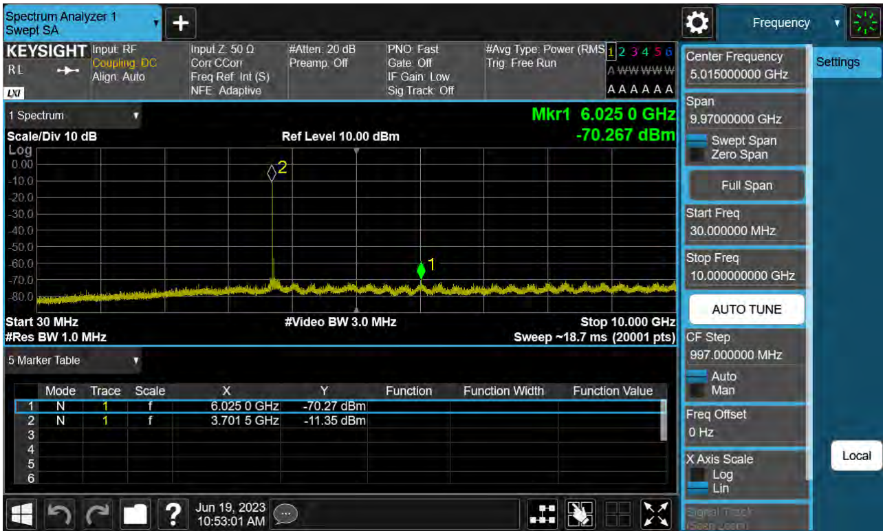
Sub6 n77. Conducted Spurious Plot_1 (648668ch_60 MHz_BPSK)
