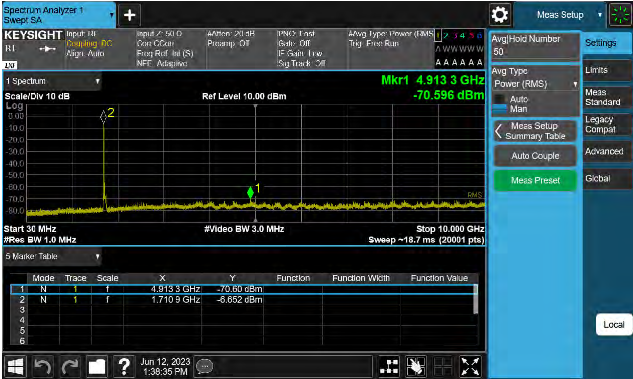
Sub6 n66. Conducted Spurious Plot_1 (345000ch_30 MHz_BPSK_RB 1_1)
