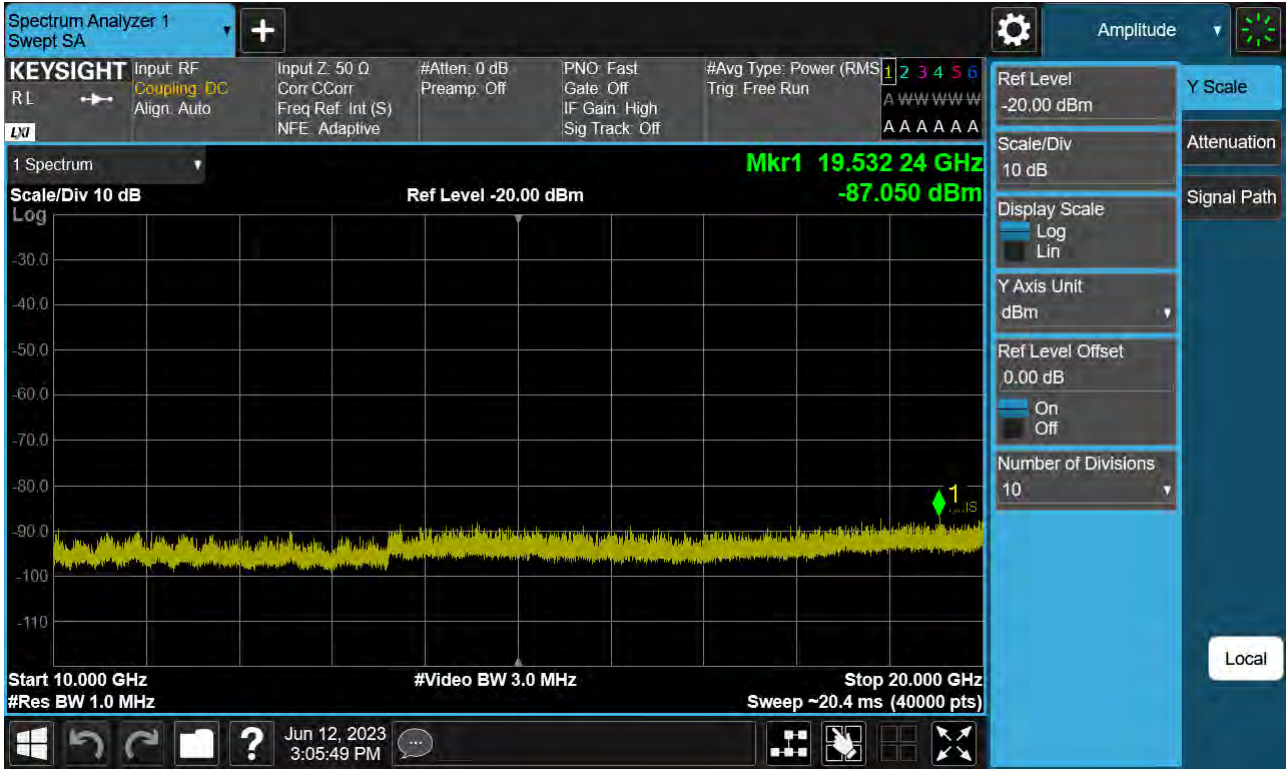
Sub6 n66. Conducted Spurious Plot_2 (349000ch_25 MHz_BPSK_RB 1_1)
