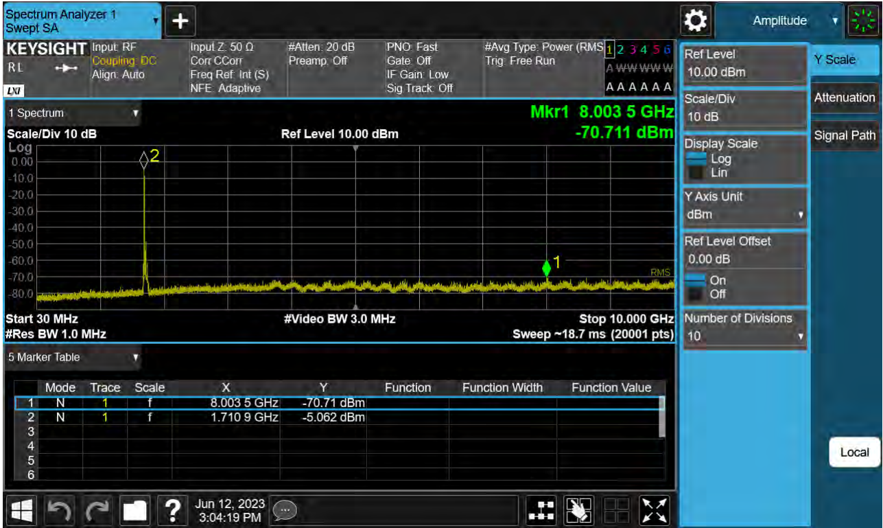
Sub6 n66. Conducted Spurious Plot_1 (344500ch_25 MHz_BPSK_RB 1_1)
