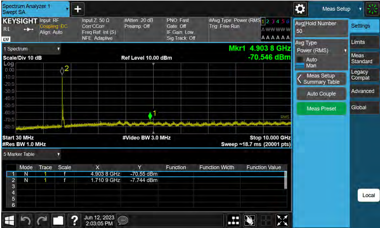
Sub6 n66. Conducted Spurious Plot_1 (346000ch_40 MHz_BPSK_RB 1_1)
