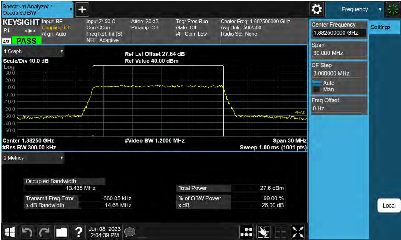
Sub6 n25(2). Occupied Bandwidth Plot (15 M BW Ch.376500 256QAM _ Full RB _0
