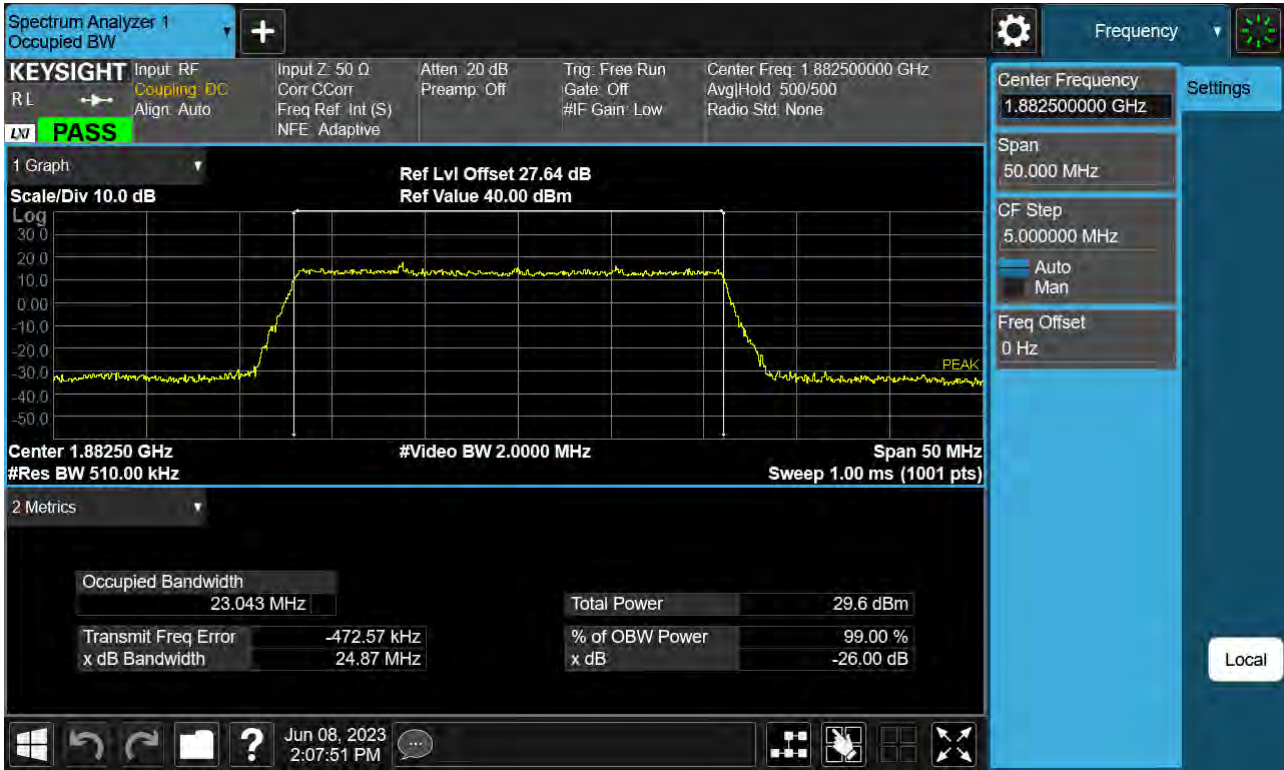
Sub6 n25(2). Occupied Bandwidth Plot (25 M BW Ch.376500 BPSK _ Full RB _0)
