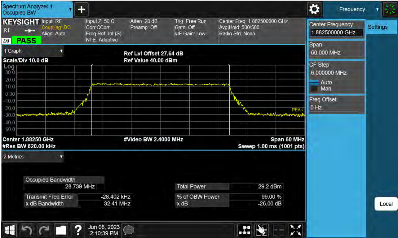
Sub6 n25(2). Occupied Bandwidth Plot (30 M BW Ch.376500 QPSK_ Full RB_0)
