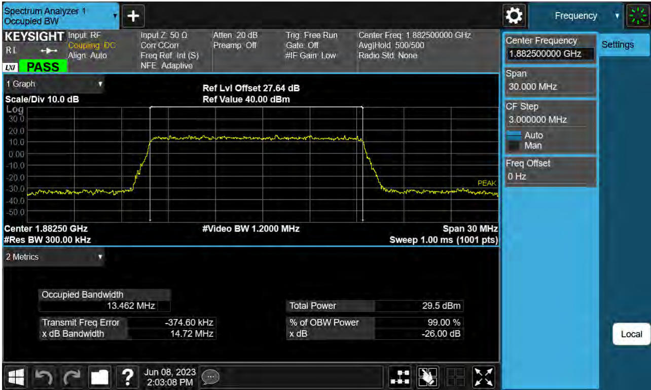
Sub6 n25(2). Occupied Bandwidth Plot (15 M BW Ch.376500 BPSK_ Full RB _0)
