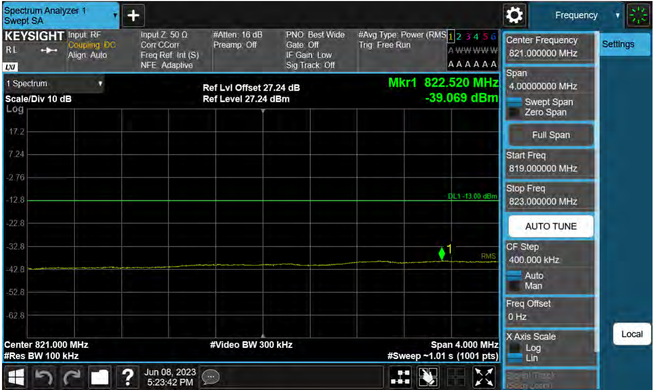
Sub6 n5. Lower Extended Band Edge Plot (20 M BW Ch.166800 BPSK_RB100_0)
