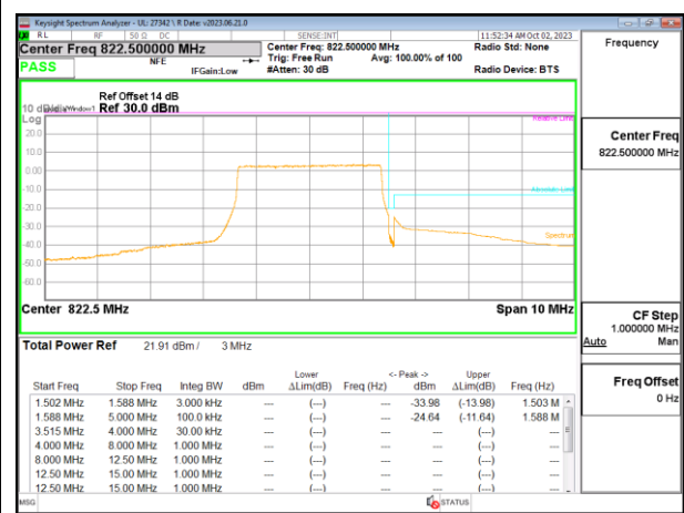
LTE B26 3MHz 16QAM High Channel RB15-0
