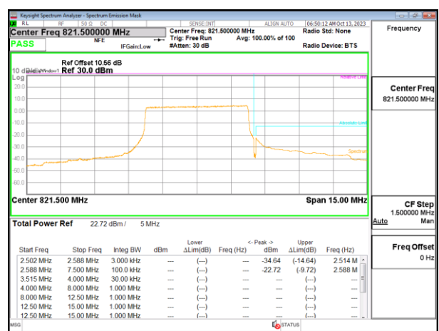
LTE B26 5MHz QPSK High Channel RB25-0
