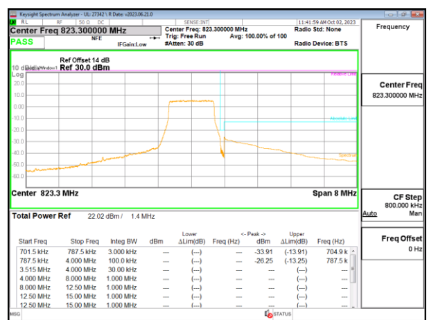
LTE B26 1.4MHz 16QAM High Channel RB6-0
