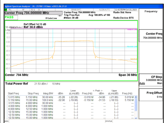
LTE B12 10MHz 16QAM Low Channel RB50-0
