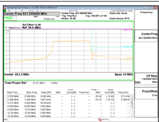
LTE B26 5MHz 16QAM High Channel RB25-0
