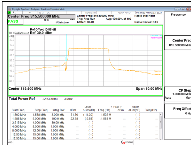
LTE B26 3MHz QPSK Low Channel RB15-0
