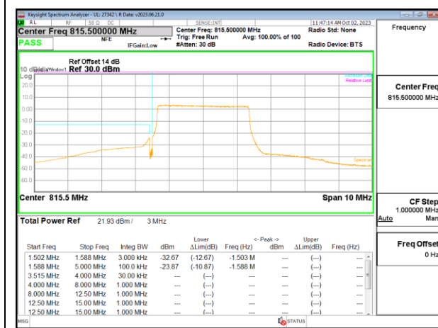
LTE B26 3MHz 16QAM Low Channel RB15-0
