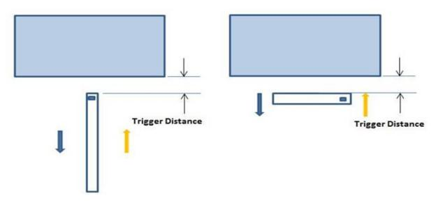
Proximity Sensor Trigger Distance Assessment KDB 616217 §6.2, Edge 3,4 Proximity Sensor Trigger Distance Assessment KDB 616217 §6.2, Rear
