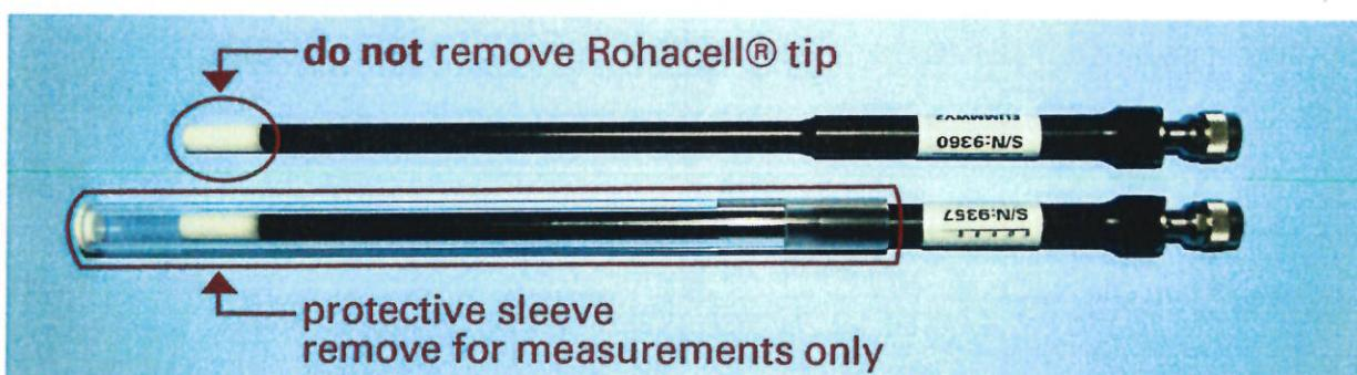
Note that probe usage is limited to free-space measurements; water, sugar-water solutions, nutrient solutions and glycol solutions will permanently damage the probe.
