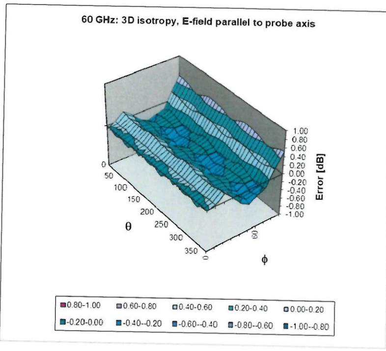
Probe isotropy for  $E_{\text{tot}}$ : probe rotated  $\varphi = 0^\circ$  to  $360^\circ$ , tilted from field propagation direction  $\bar{k}$
