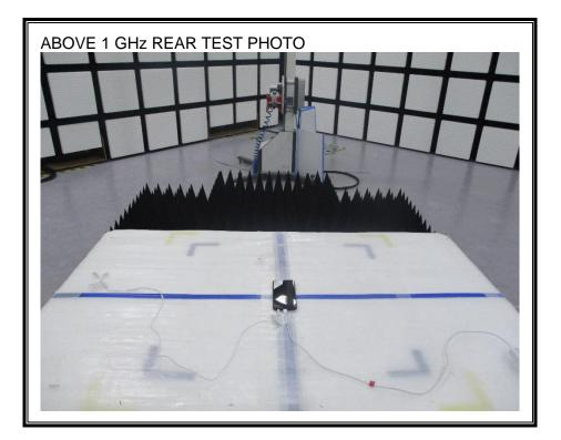
5) RADIATED RF MEASUREMENT SET-UP (Axis)
