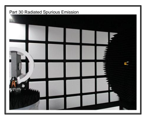
4) <u>RADIATED RF MEASUREMENT SETUP (WWAN Receiver mode)</u>
