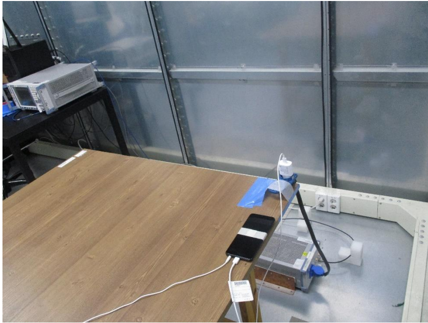
AC LINE CONDUCTED FRONT TEST PHOTO
