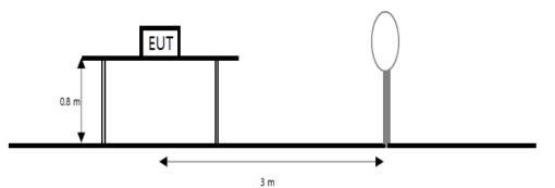
The diagram below shows the test setup that is utilized to make the measurements for emission from 30 Mb to 1 Gb emissions.
