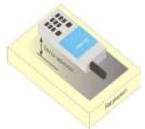
Figure 8-6 Sample Body-Worn Diagram
