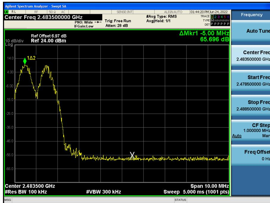
Test Plots with hopping (8DPSK)
