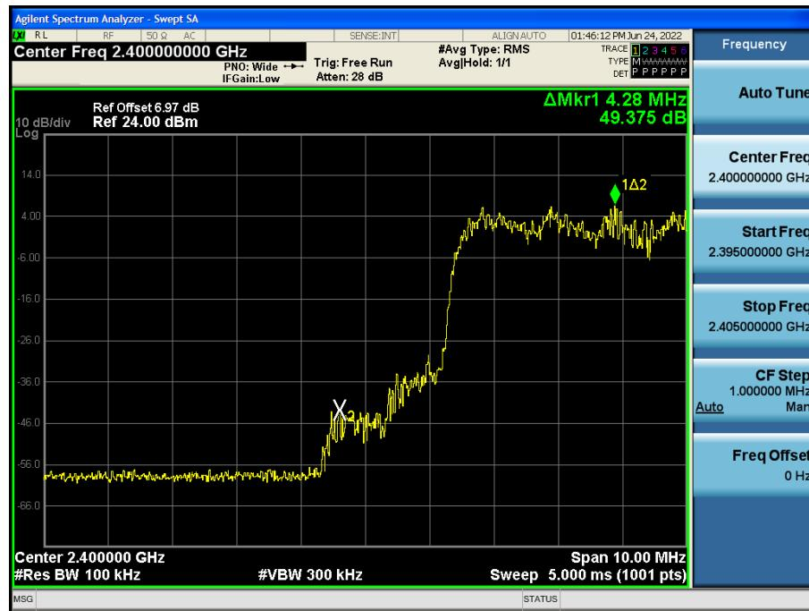
Test Plots with hopping (8DPSK)
