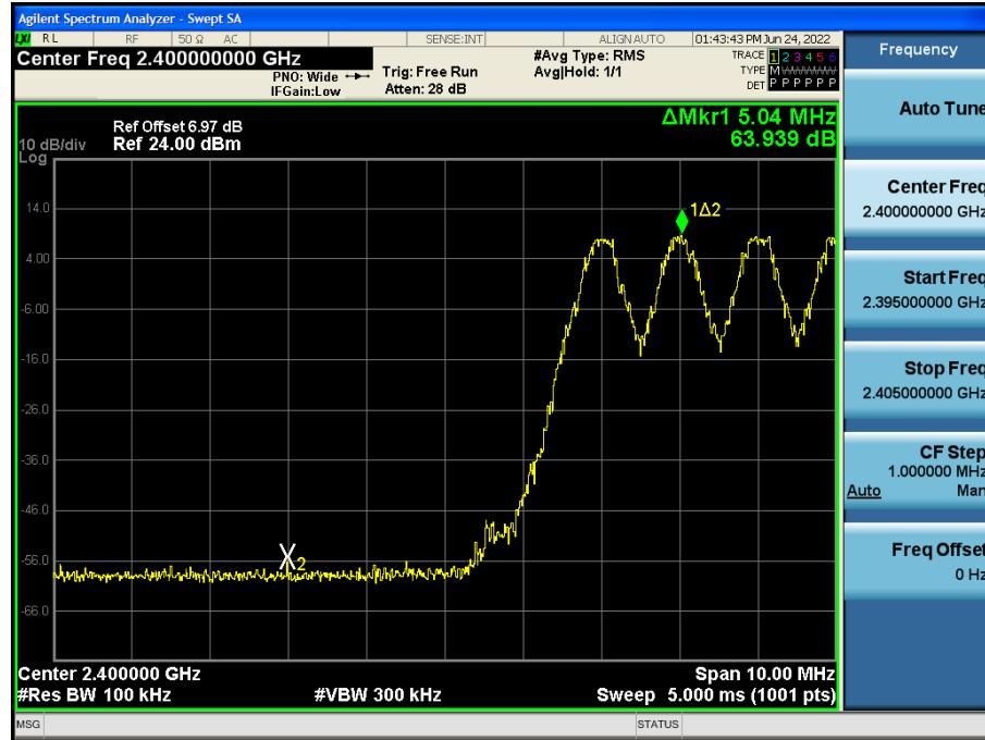
Test Plots with hopping (GFSK)
