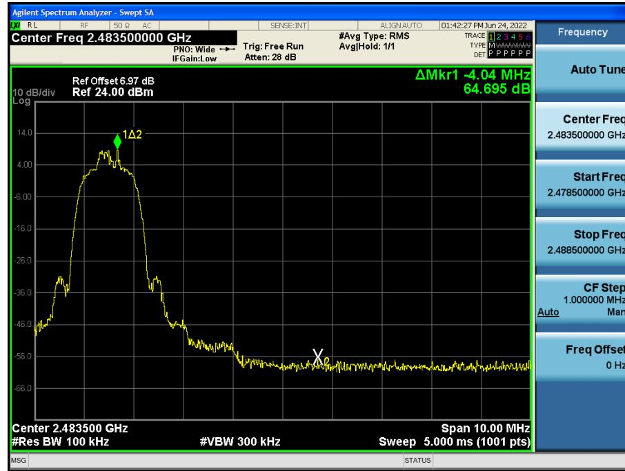
Test Plots with hopping (GFSK)
