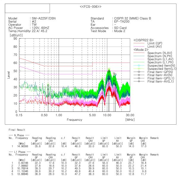
Note 1) Two graphs measured for both Live(L1) and Neutral(N) of the LISN are combined into one graph Note 2) Level (QP and/or CAV) = Meter Reading (QP and/or CAV) + Corr. (LISN Insertion Loss + Cable Loss) Margin (QP and/or CAV) = Limit – Level (QP and/or CAV) QP = Quasi-Peak, CAV = CISPR-Average, Corr. = Correction Factor.
