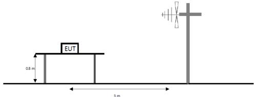
The diagram below shows the test setup that is utilized to make the measurements for emission from 1  $\mathbb{G}$  to the tenth harmonic of the highest fundamental frequency or to 40  $\mathbb{G}$  emissions, whichever is lower.
