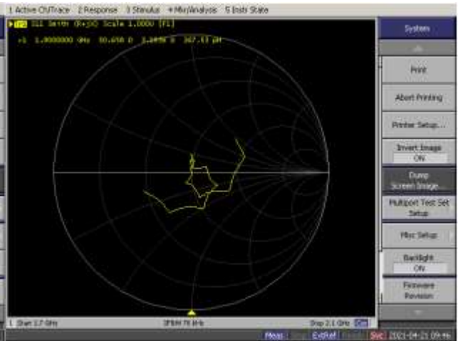
< Figure 2. Measurement result of Head Impedance >
