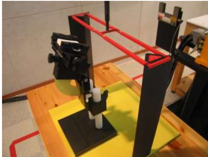
Figure 2. HAC Phantom & Device Holder
