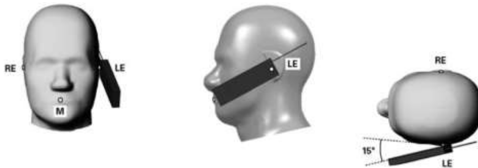
Figure 8.5. Tilt 15° position of the wireless device
