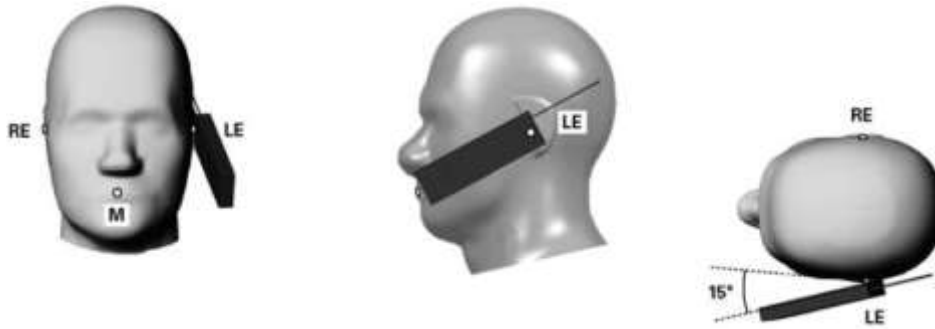
Figure 8.5. Tilt 15° position of the wireless device
