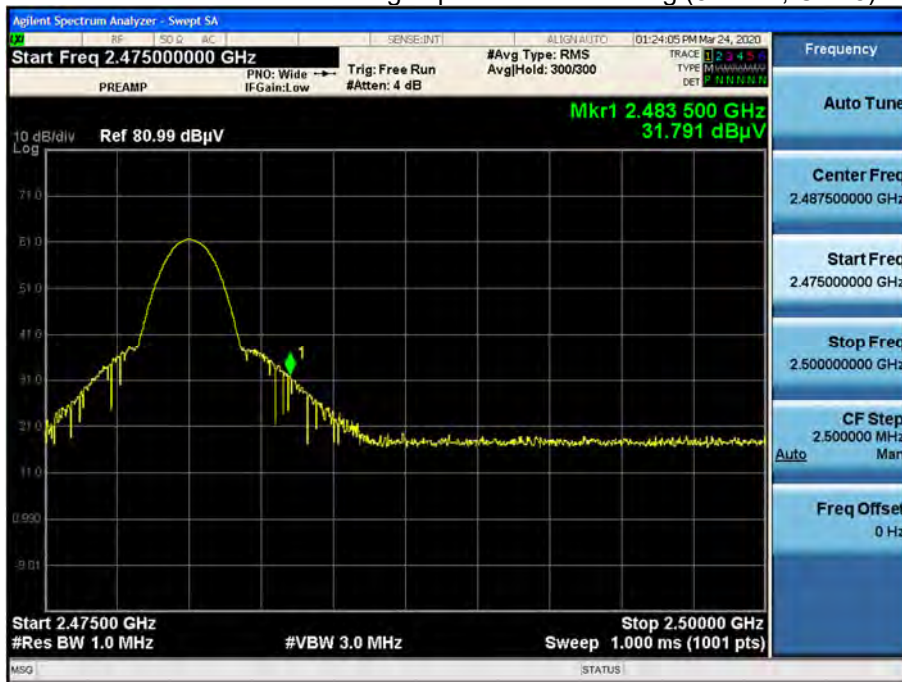
Radiated Restricted Band Edges plot – Peak Reading (8DPSK, Ch.78)
