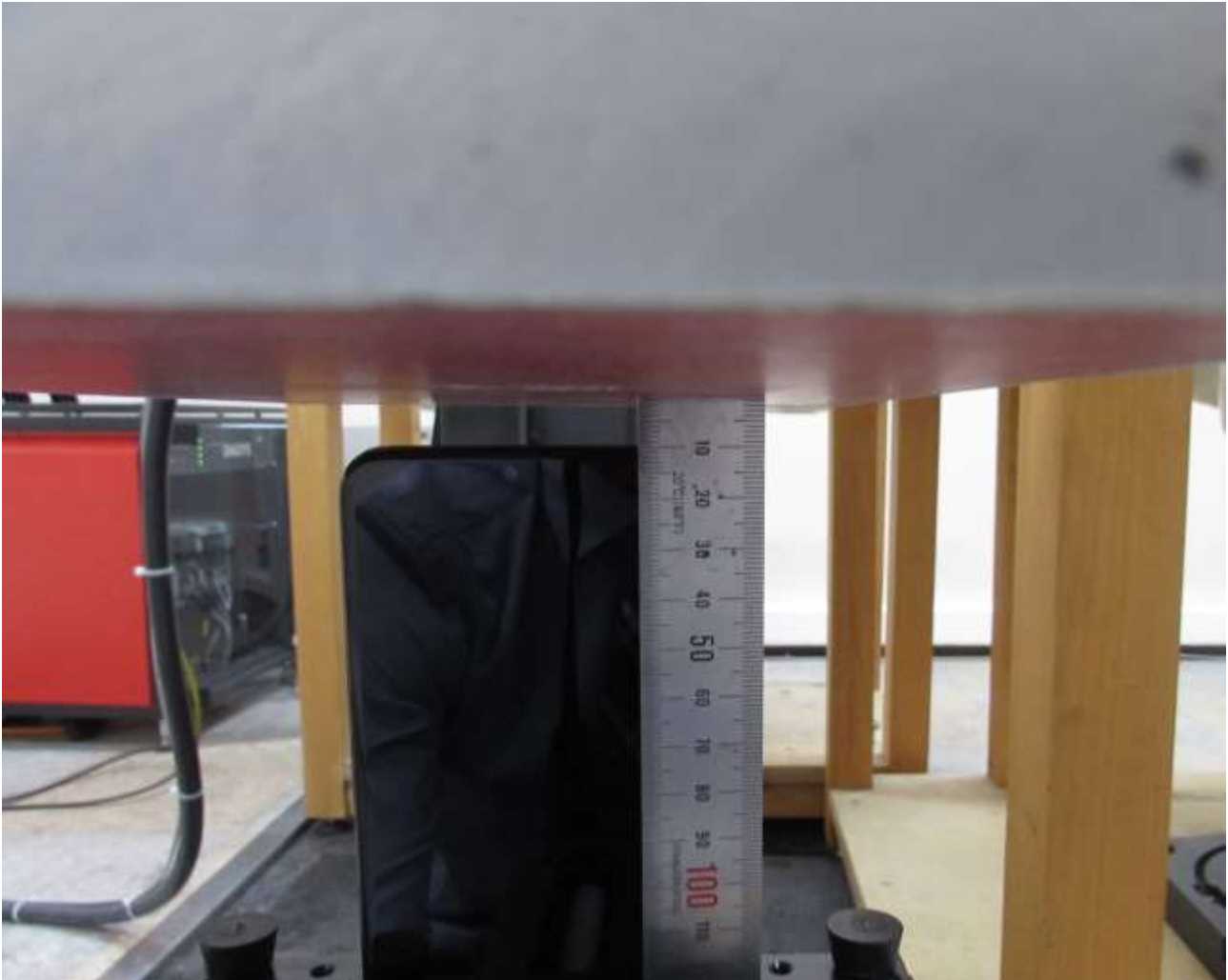
[Distance of 10 mm from the EUT]
