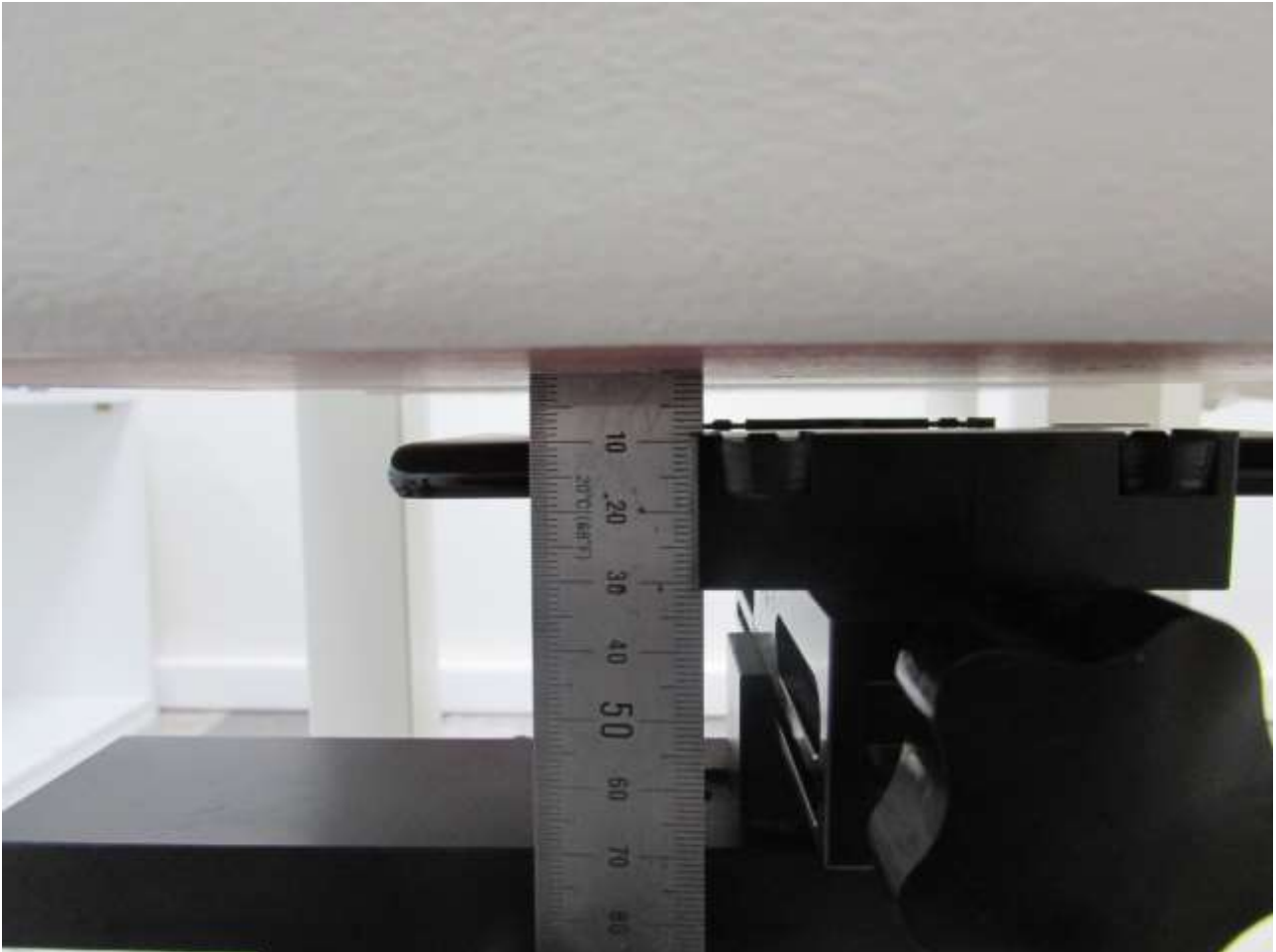
[Distance of 10 mm from the EUT]
