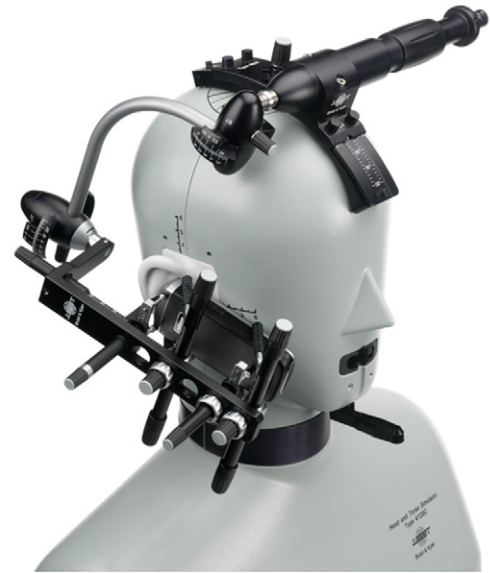
Figure 4-3 Heat and Torso Simulator (with Handset Positioner)
