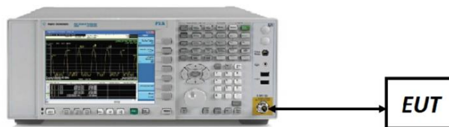
Figure 7-5. Test Instrument & Measurement Setup
