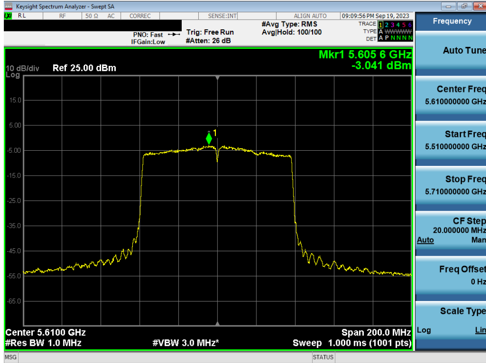
Plot 7-28. Power Spectral Density Plot (80MHz BW 802.11ac (UNII Band 2C) – Ch. 122)
