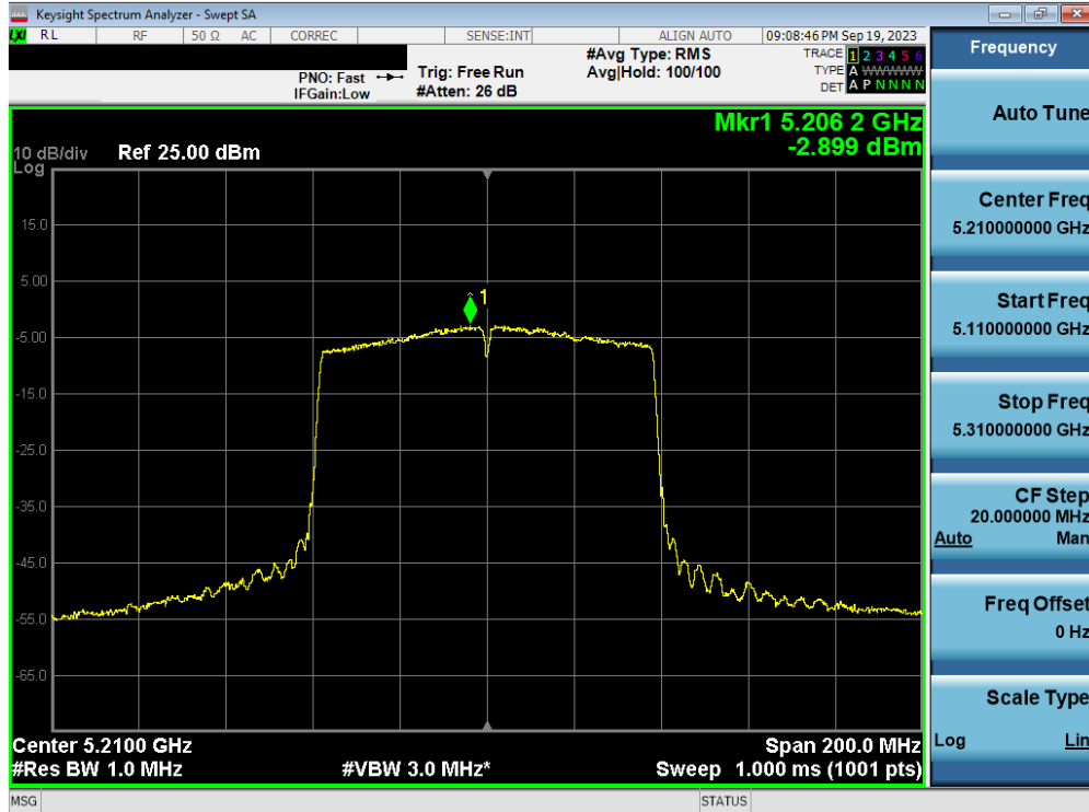
Plot 7-20. Power Spectral Density Plot (80MHz BW 802.11ac (UNII Band 1) – Ch. 42)
