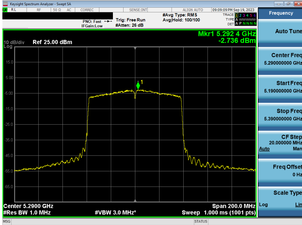
Plot 7-24. Power Spectral Density Plot (80MHz BW 802.11ac (UNII Band 2A) – Ch. 58)
