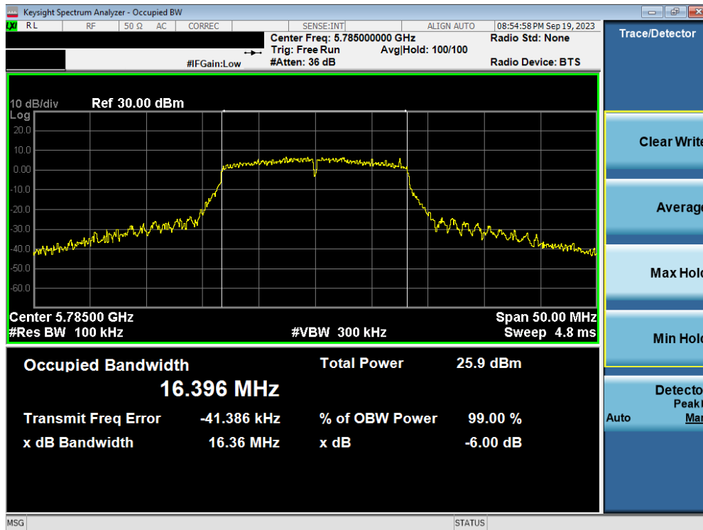
Plot 7-13. 6dB Bandwidth Plot (802.11a (UNII Band 3) – Ch. 157)
