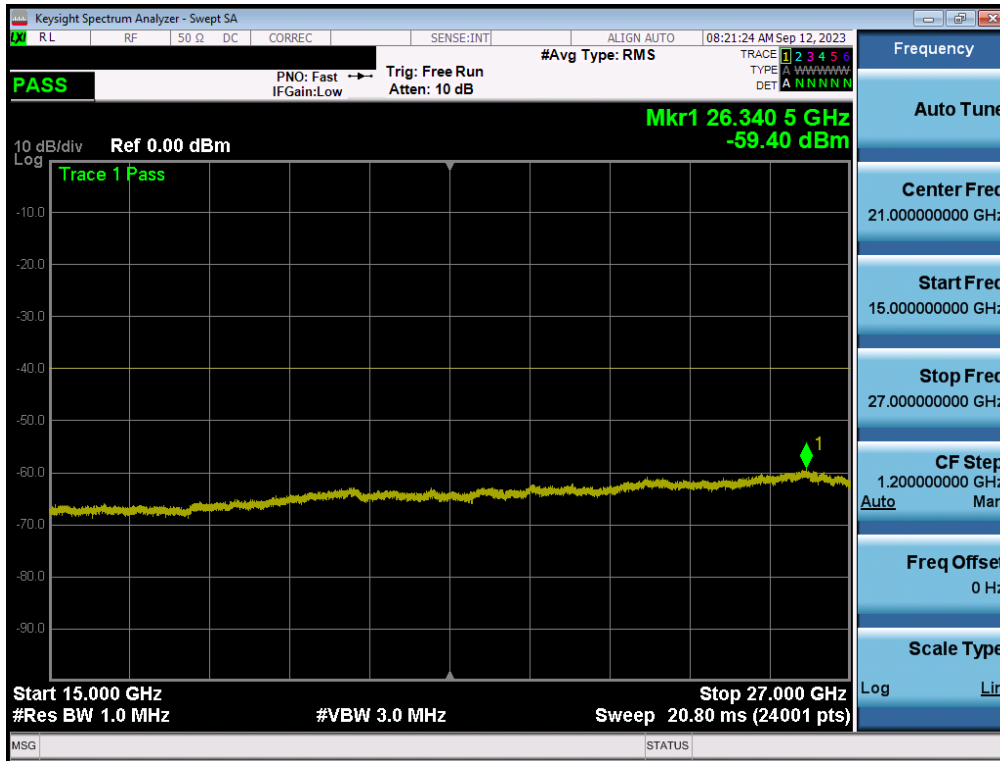
Plot 7-68. Conducted Spurious Plot (LTE Band 30 - 10MHz QPSK - RB Size 1, RB Offset 0)
