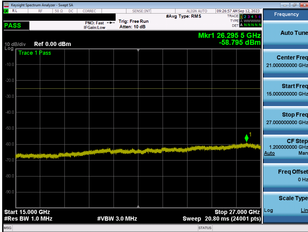
Plot 7-71. Conducted Spurious Plot (LTE Band 7 - 20MHz QPSK - RB Size 1, RB Offset 0 - High Channel)
