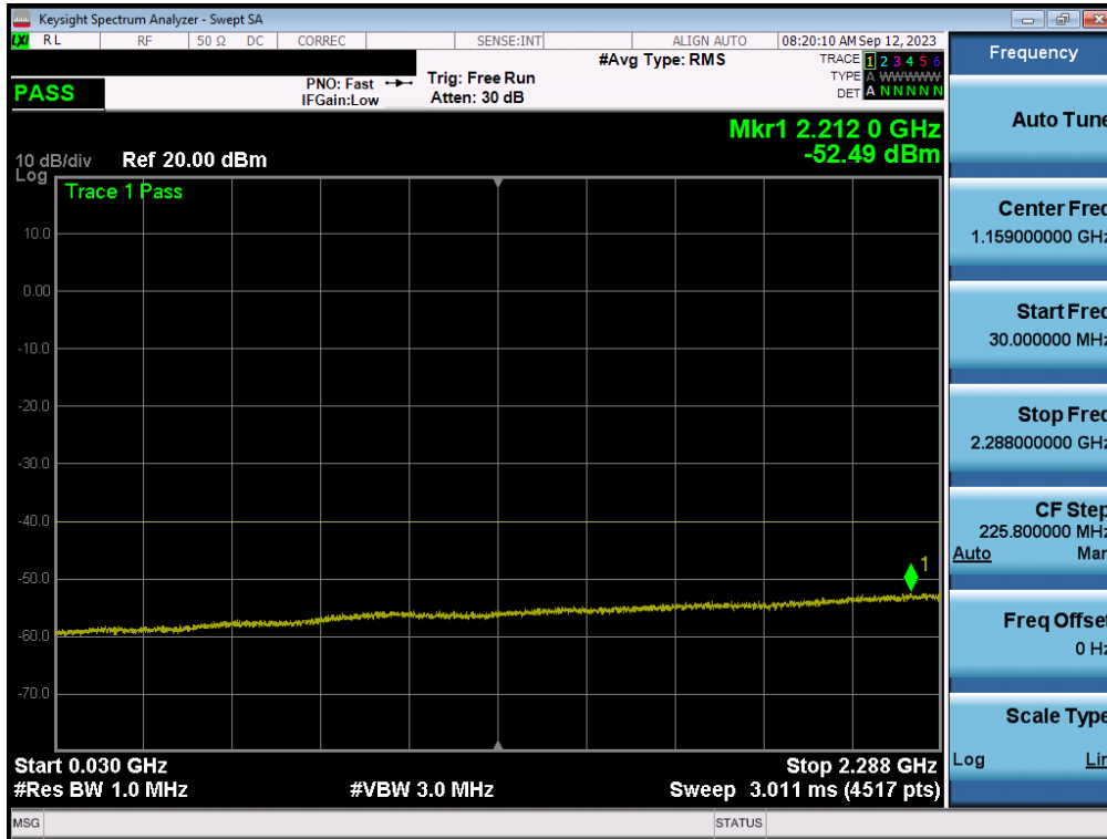
Plot 7-66. Conducted Spurious Plot (LTE Band 30 - 10MHz QPSK - RB Size 1, RB Offset 0)
