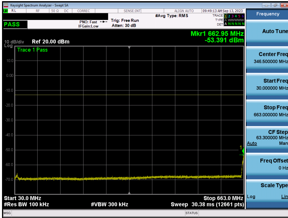
Plot 7-109. Conducted Spurious Plot (LTE Band 71 - 20MHz QPSK - 1 RB - High Channel - ANT1)
