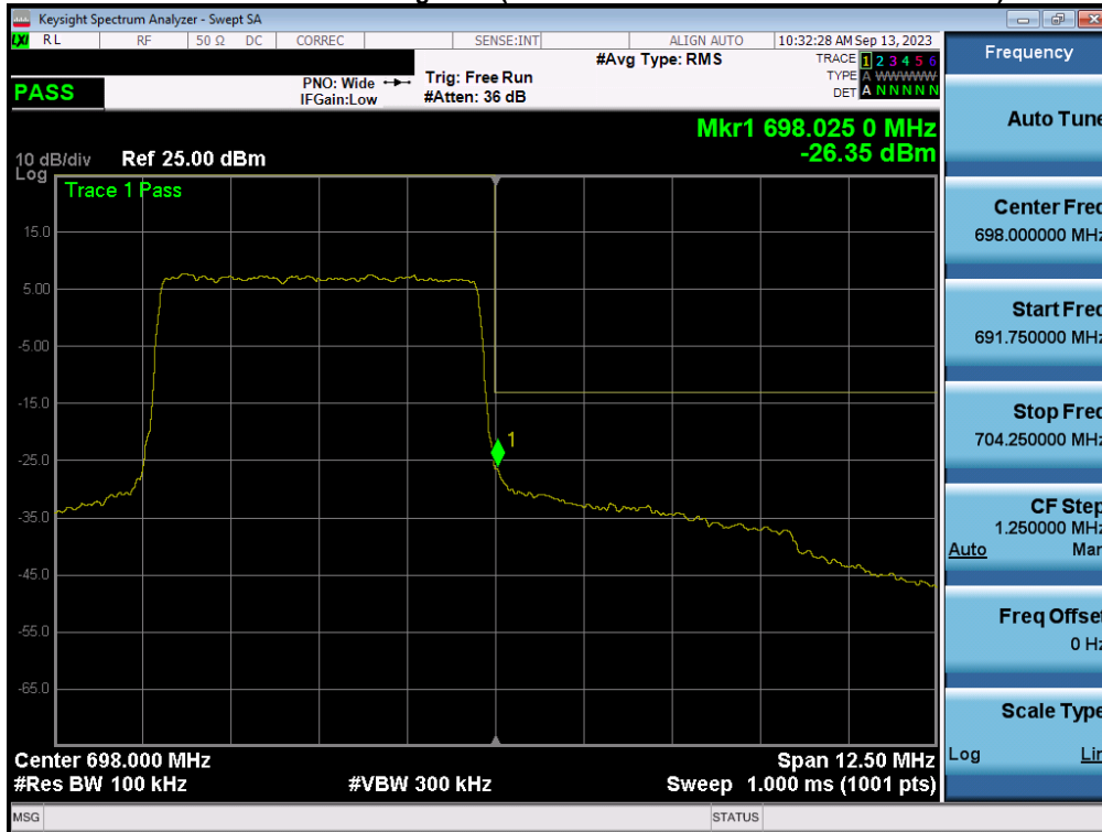
Plot 7-140. Upper Band Edge Plot (LTE Band 71 - 5MHz QPSK – Full RB - ANT1)
