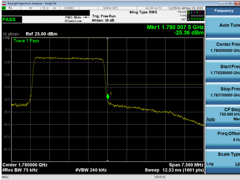
Plot 7-157. Upper Band Edge Plot (LTE Band 66 - 3MHz QPSK – Full RB - ANT1)
