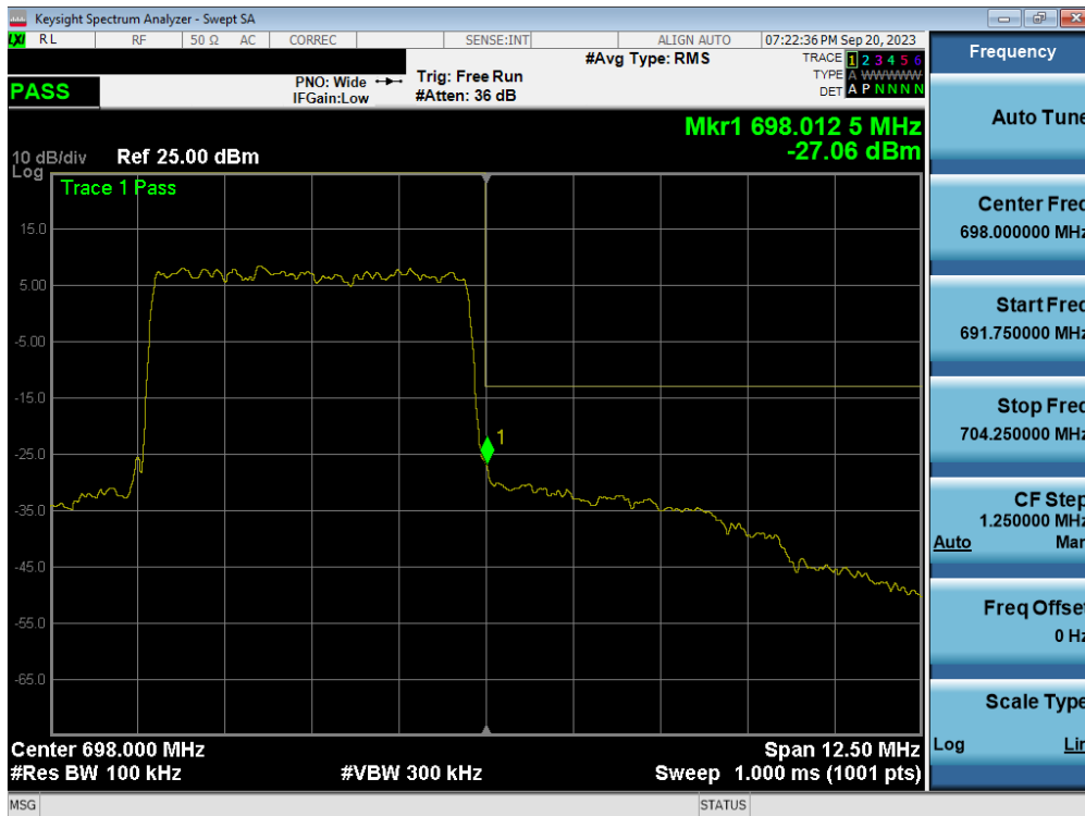
Plot 7-148. Upper Band Edge Plot (NR Band n71 – 5.0MHz - Full RB - ANT1)
