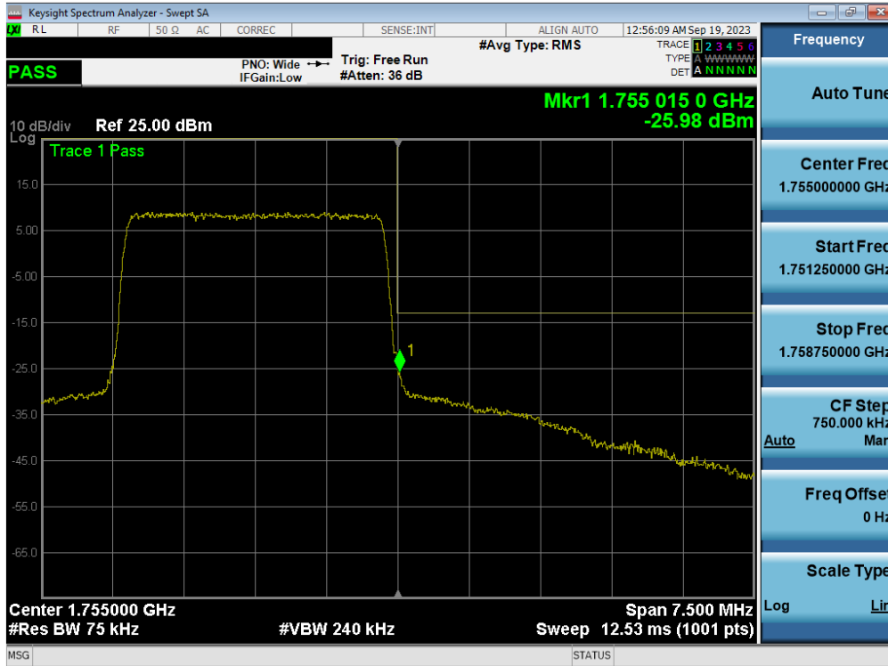
Plot 7-155. Upper Band Edge Plot (LTE Band 4 - 3MHz QPSK – Full RB - ANT1)
