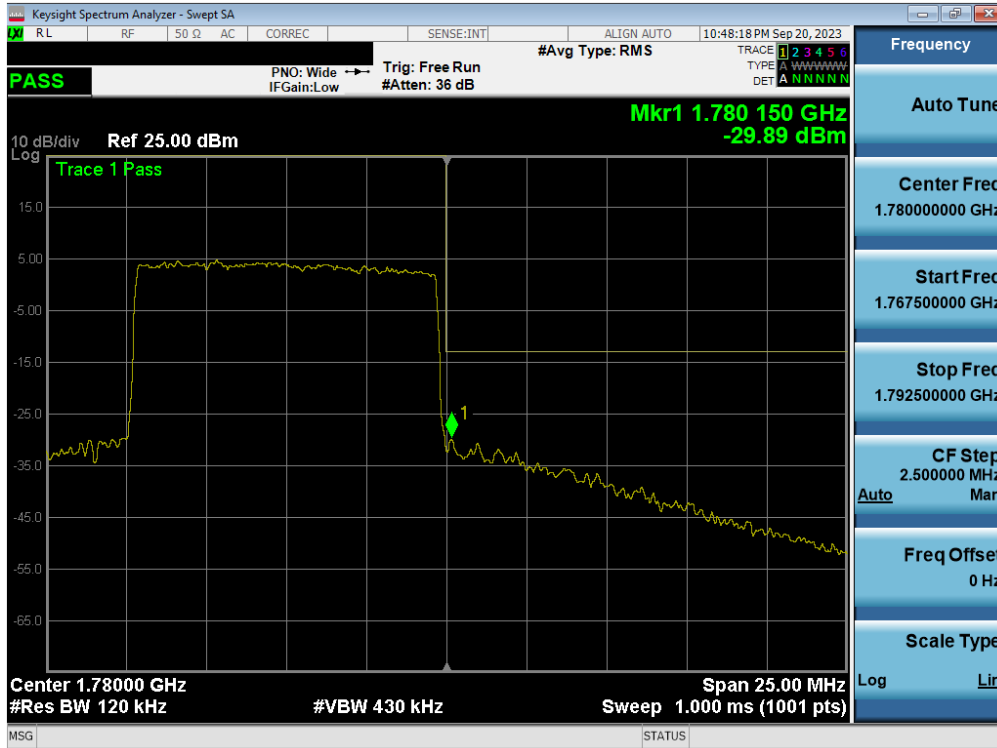
Plot 7-165. Upper Band Edge Plot (NR Band n66 – 10.0MHz - Full RB - ANT1)
