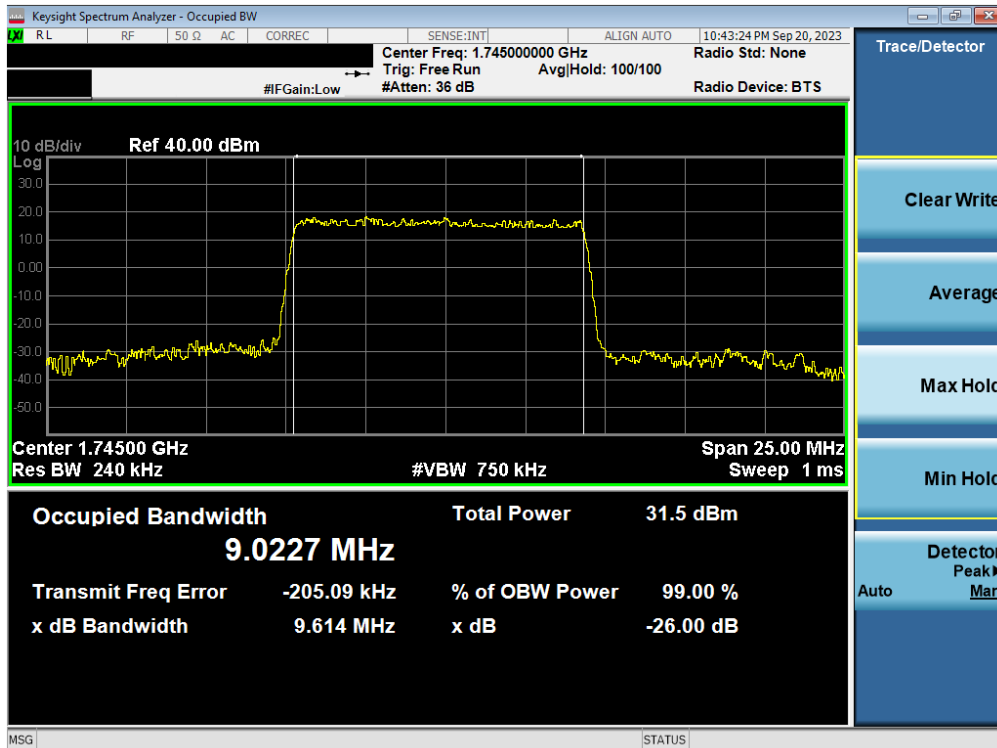
Plot 7-61. Occupied Bandwidth Plot (NR Band n66 - 10.0MHz DFT-s-OFDM BPSK - Full RB – ANT1)
