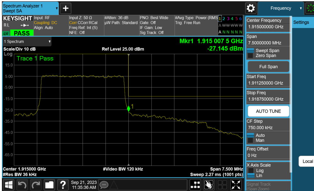
Plot 7-100. Upper Band Edge Plot (LTE Band 25 - 3MHz QPSK – Full RB - Ant M2)
