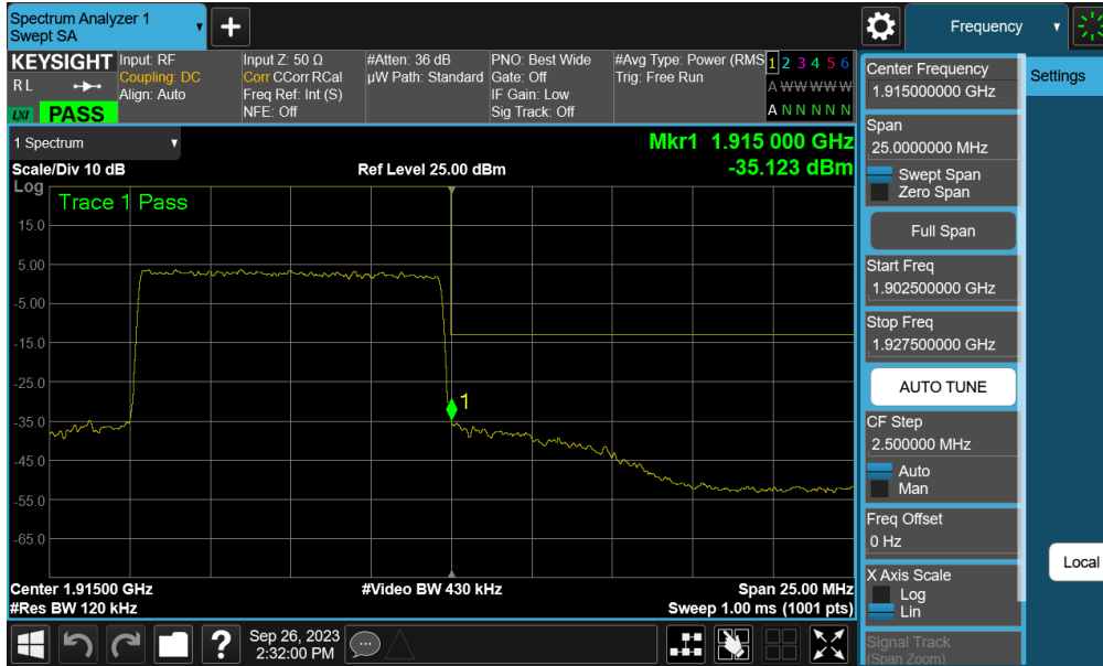
Plot 7-106. Upper Band Edge Plot (NR Band n25 - 10MHz QPSK – Full RB - Ant M2)
