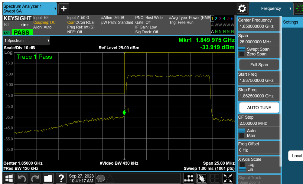
Plot 7-114. Lower Band Edge Plot (NR Band n2 - 10MHz QPSK – Full RB - Ant M3)
