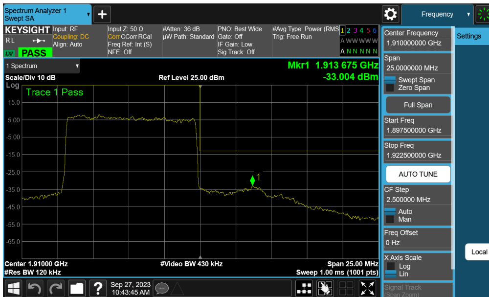
Plot 7-116. Upper Band Edge Plot (NR Band n2 - 10MHz BPSK – Full RB - Ant M3)
