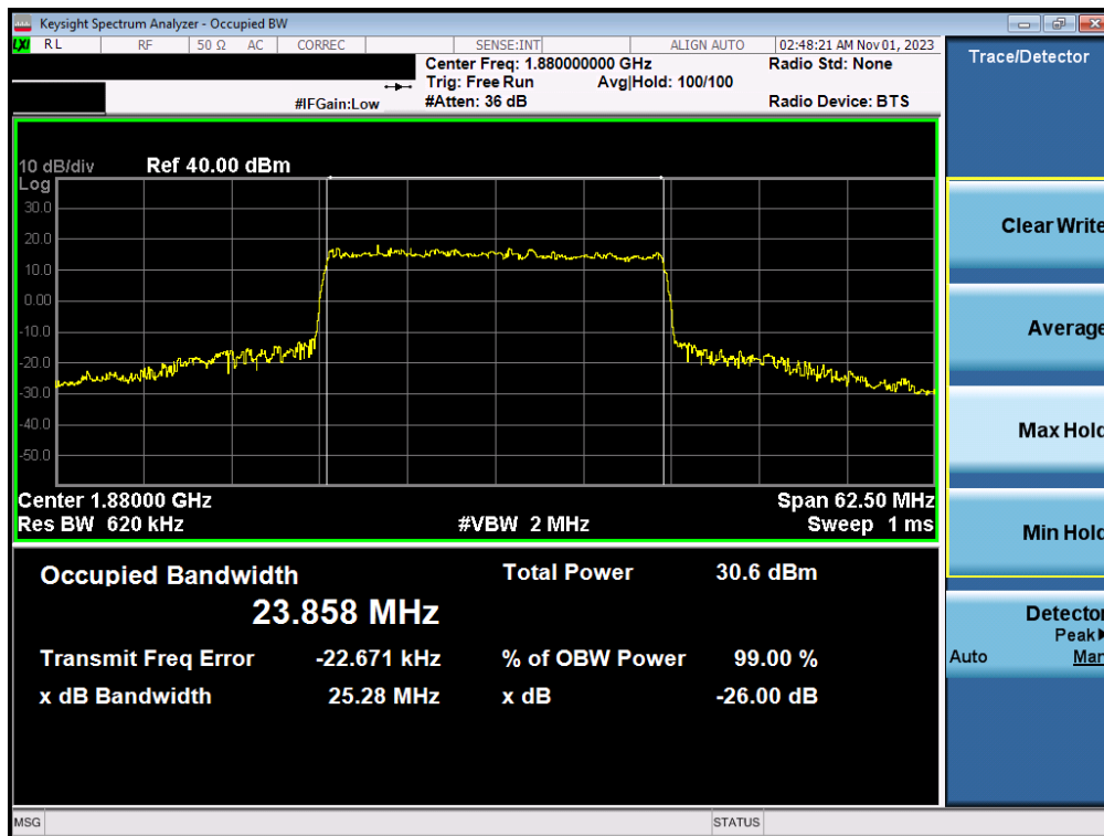
Plot 7-56. Occupied Bandwidth Plot (NR Band n2 - 25.0MHz CP-OFDM QPSK - Full RB - ANT M3)
