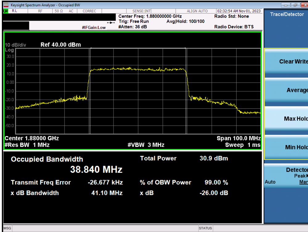
Plot 7-51. Occupied Bandwidth Plot (NR Band n2 - 40.0MHz CP-OFDM 16QAM - Full RB - ANT M3)
