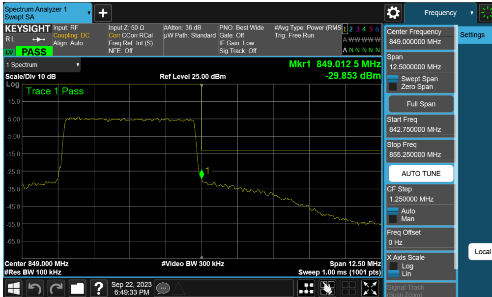
Plot 7-41. Upper Band Edge Plot (NR Band n5 – 5.0MHz CP - Full RB)
