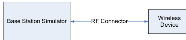
Figure 10-4 Power Measurement Setup – NR FDD
