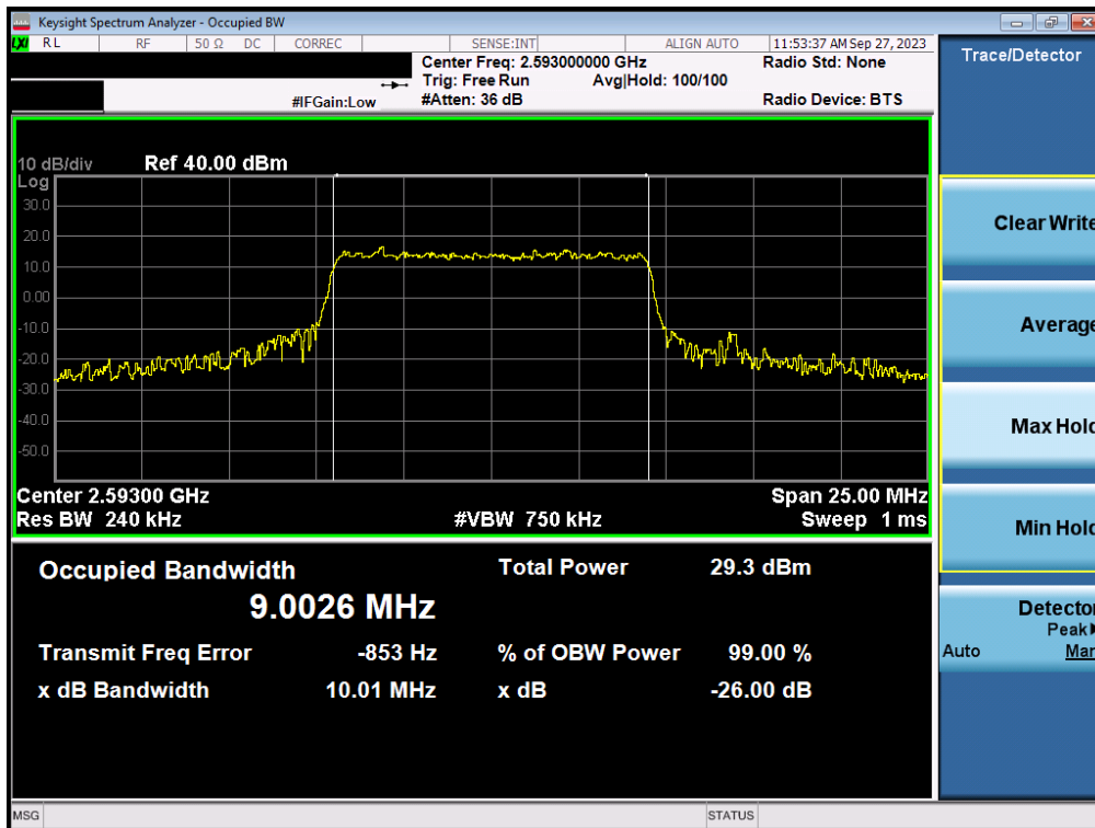
Plot 7-7. Occupied Bandwidth Plot (LTE Band 41(PC3) - 10MHz 16-QAM - Full RB)
