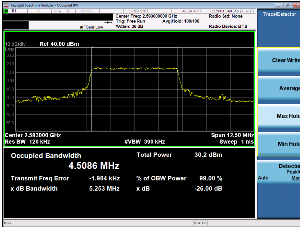
Plot 7-8. Occupied Bandwidth Plot (LTE Band 41(PC3) - 5MHz QPSK - Full RB)
