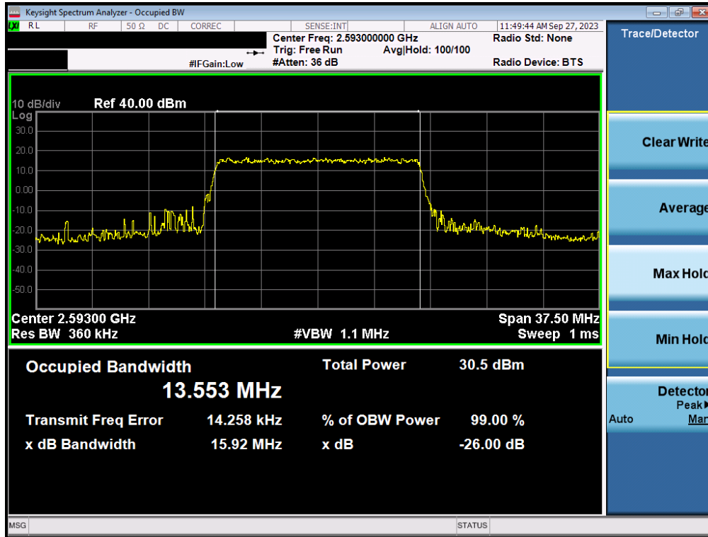
Plot 7-4. Occupied Bandwidth Plot (LTE Band 41(PC3) - 15MHz QPSK - Full RB)
